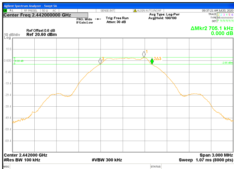
Figure 6: DTS Bandwidth-Headset -2442 MHz
