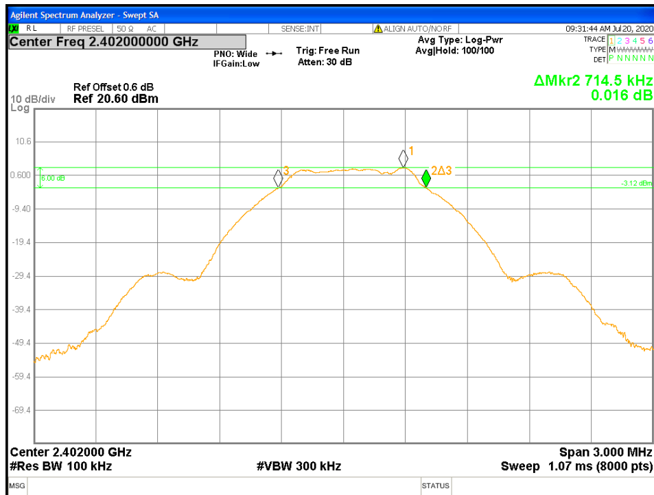
Figure 5: DTS Bandwidth-Headset -2402 MHz
