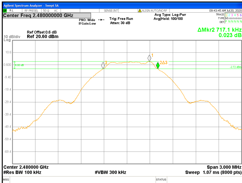
Figure 7: DTS Bandwidth-Headset -2480 MHz
