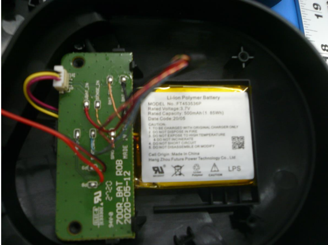
Figure 4: Internal Photo of Stealth 700P Gen 2 RX – Right Ear PCB and Battery
