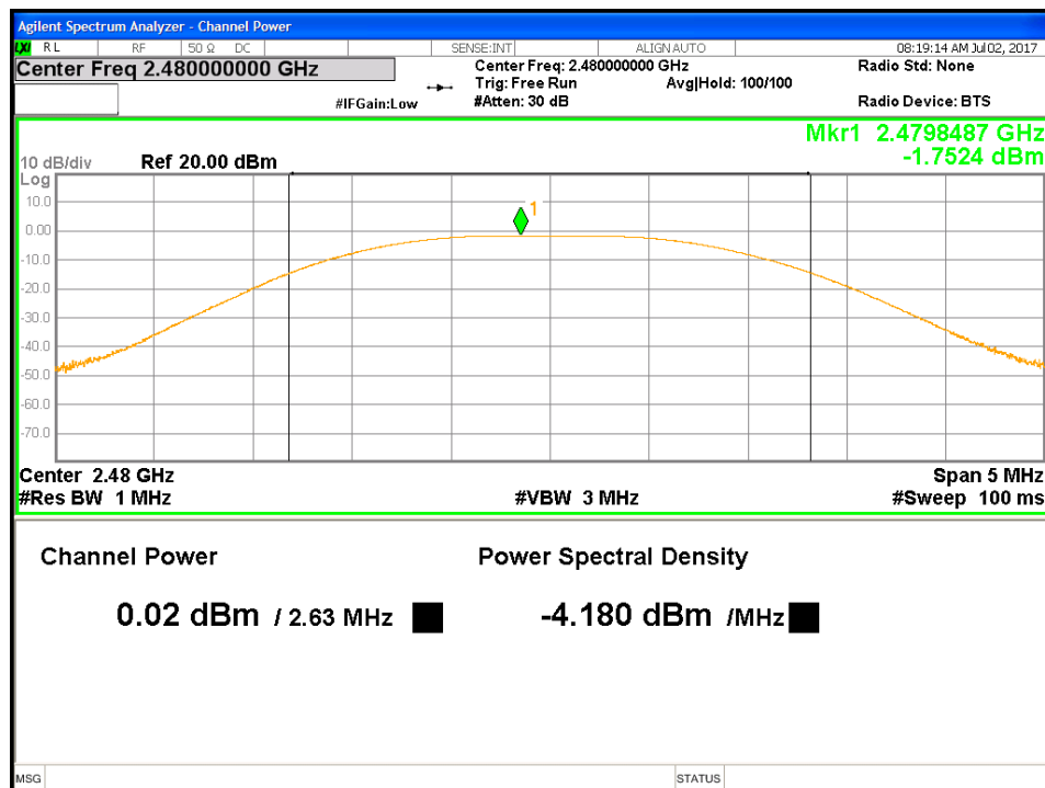
Figure 12: Maximum Transmitted Power at 2480 MHz, BLE
