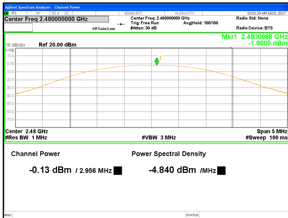
Figure 6: Maximum Transmitted Power at 2480 MHz, 2DH1
