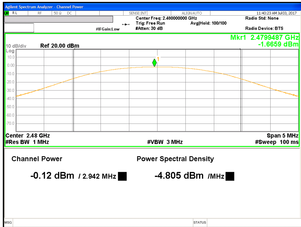
Figure 9: Maximum Transmitted Power at 2480 MHz, 3DH3
