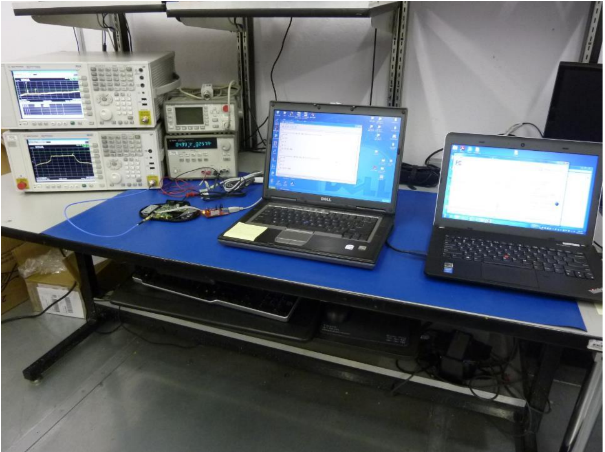
Figure 7: RF Conducted Test Setup
