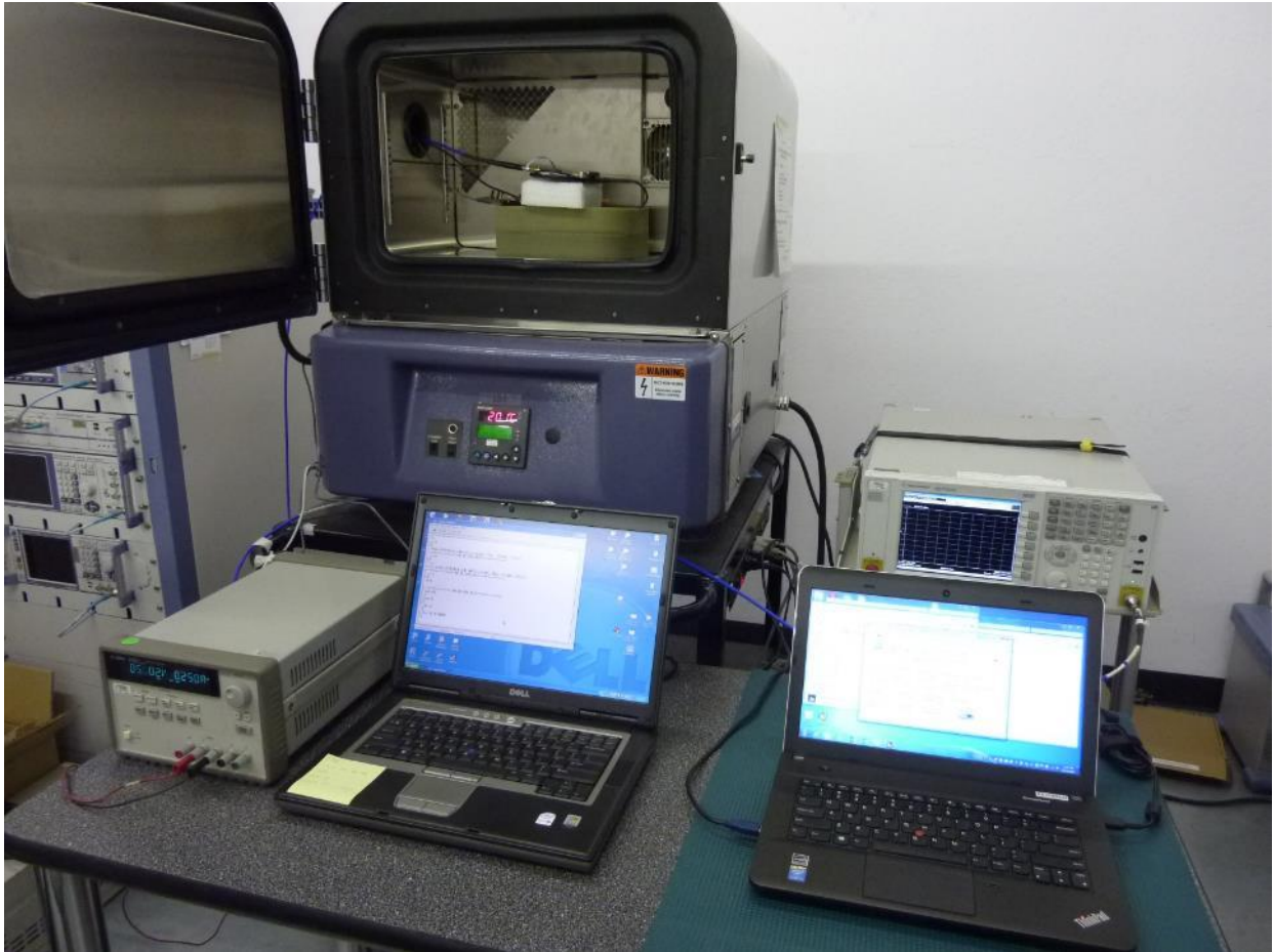
Figure 9: Frequency Stability Test Setup (Outside Thermo Chamber)
