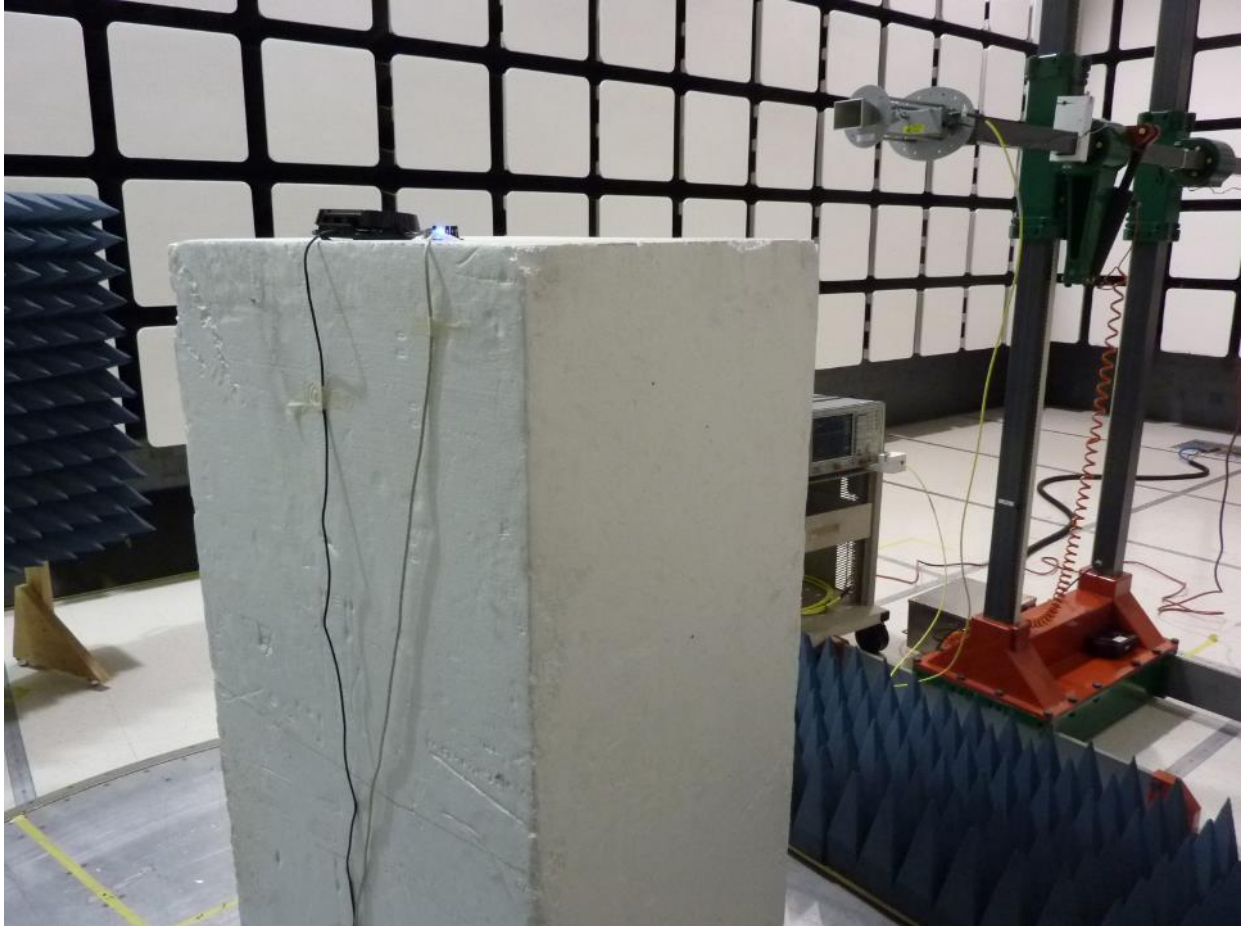
Figure 6: Test Setup for 18 GHz to 40GHz (Rear View)
