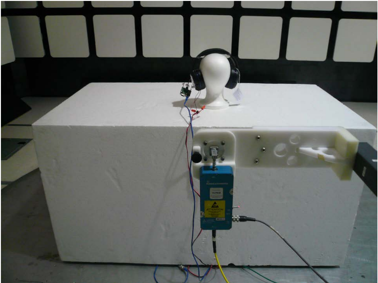
Figure 6: Test Setup for 18 GHz to 26GHz (Rear View)
