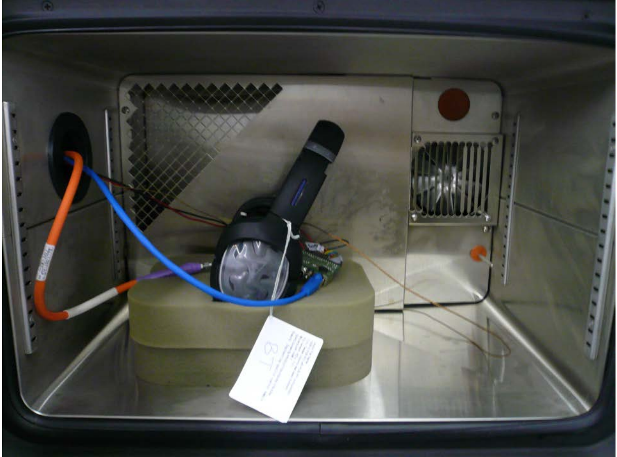
Figure 12: Frequency Stability Test Setup (Inside Thermo Chamber)
