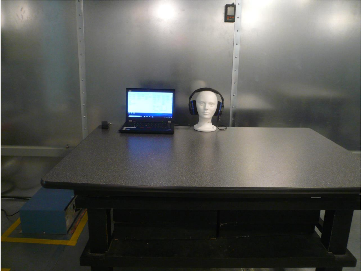
Figure 10: AC Conducted Emission Test Setup (Front)
