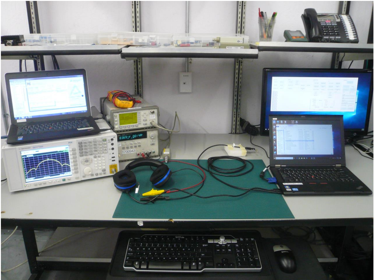
Figure 9: RF Conducted Test Setup
