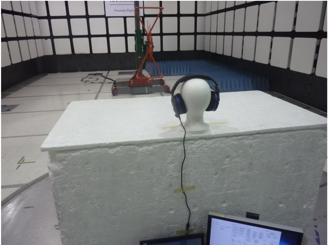
Figure 3: Test Setup for 30 MHz to 1000 MHz (Front View)
