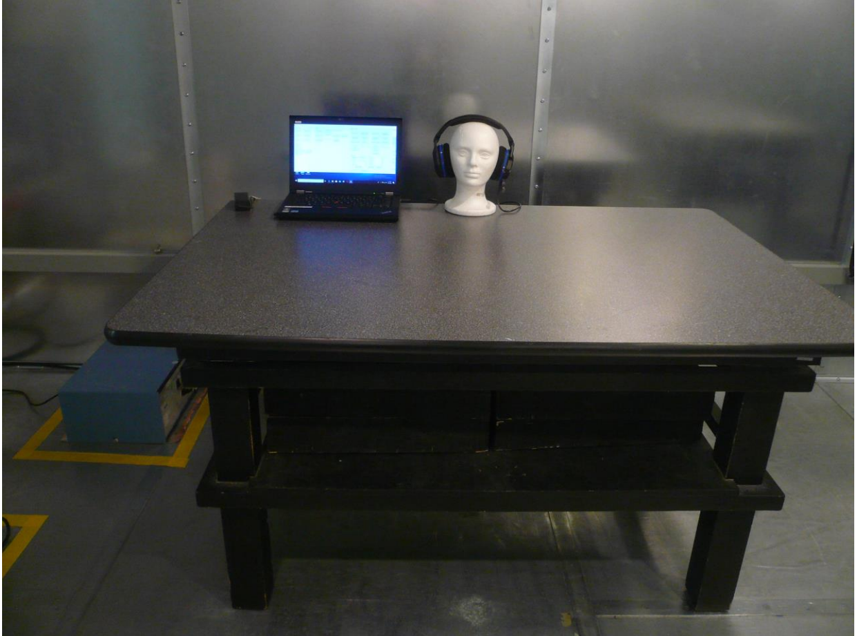
Figure 10: AC Conducted Emission Test Setup (Front View)
