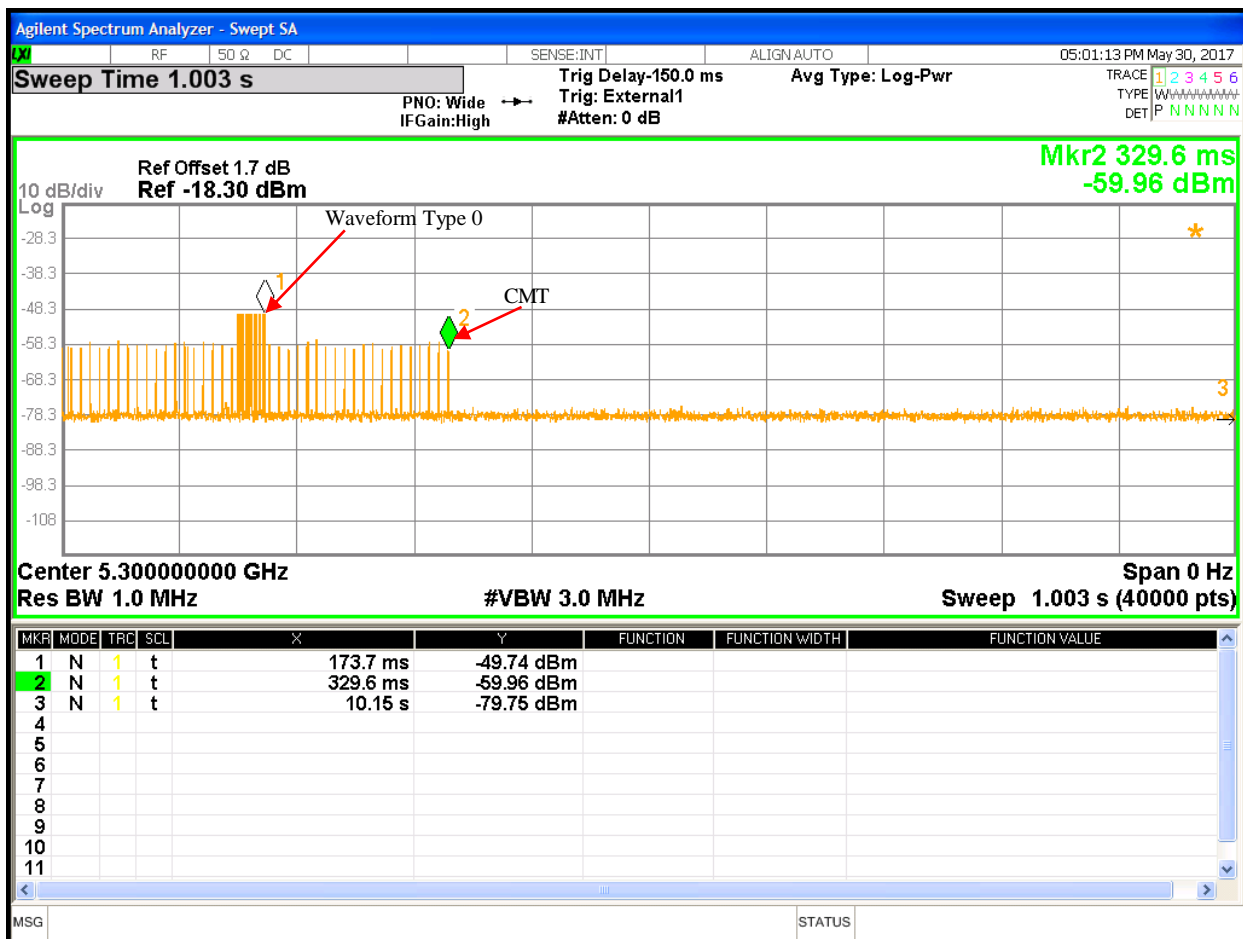
Figure 4: Channel Move Time and Channel Closing Transmission Time using Pulse Radar Waveform 0 at 5300 MHz, 20 MHz Bandwidth (Close-up)
