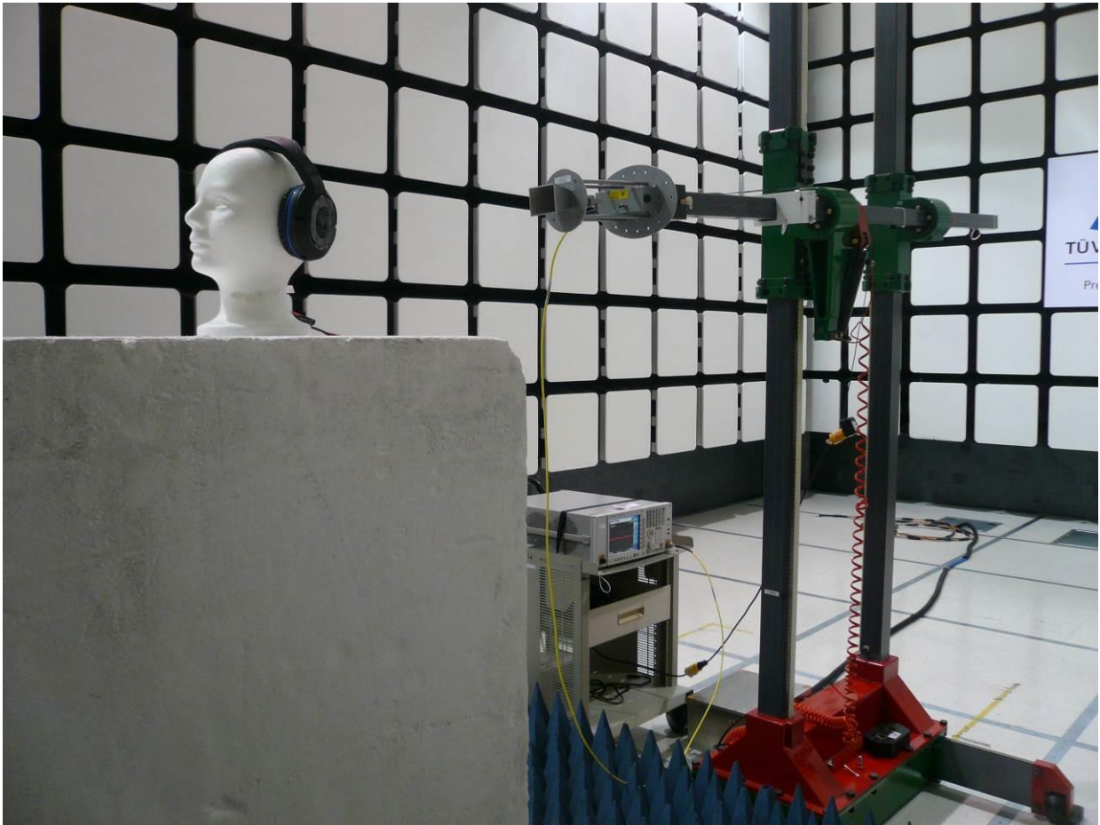
Figure 5: Test Setup for 18 GHz to 26 GHz (Front View) – Y-Axis
