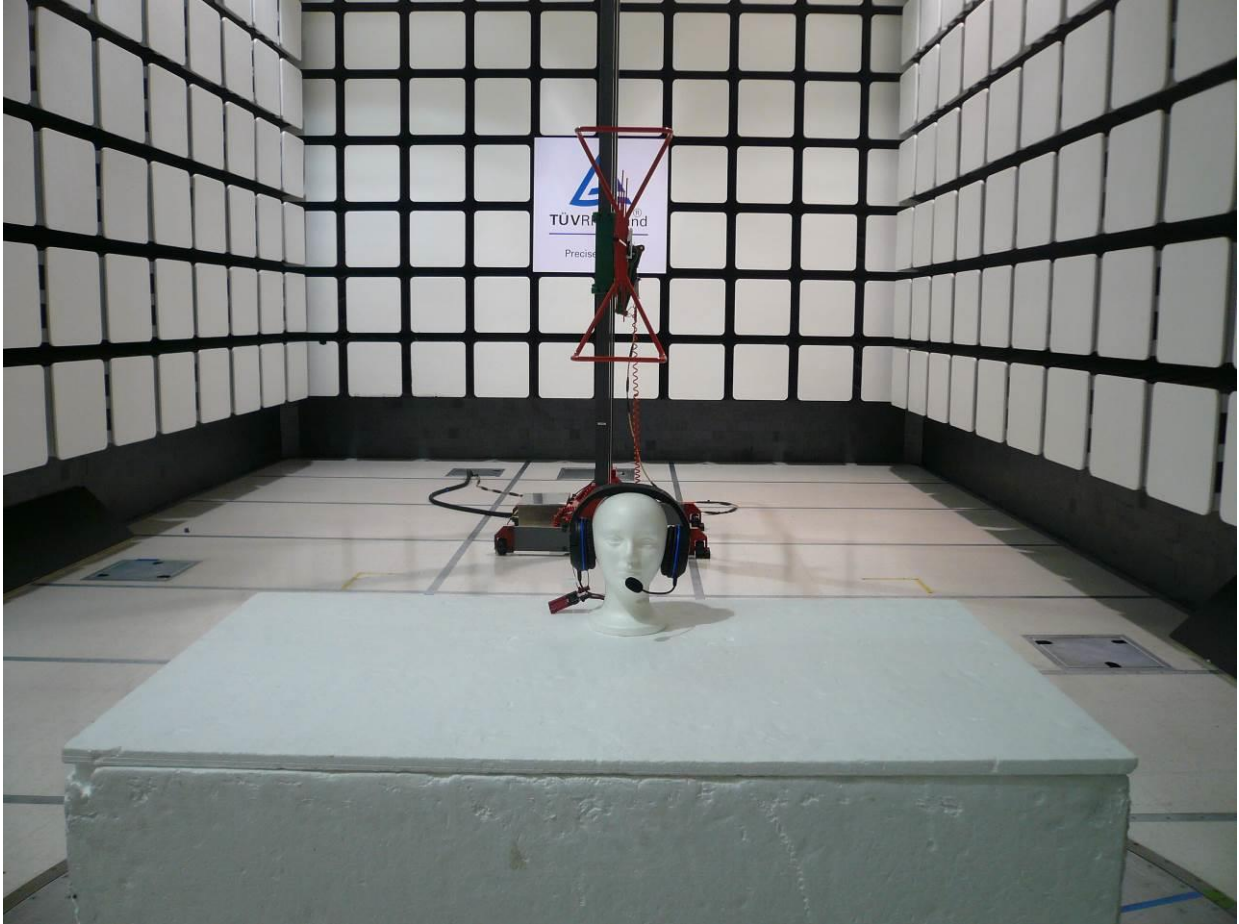
Figure 1: Test Setup for 30 MHz to 1000 MHz (Front View) – Y-Axis
