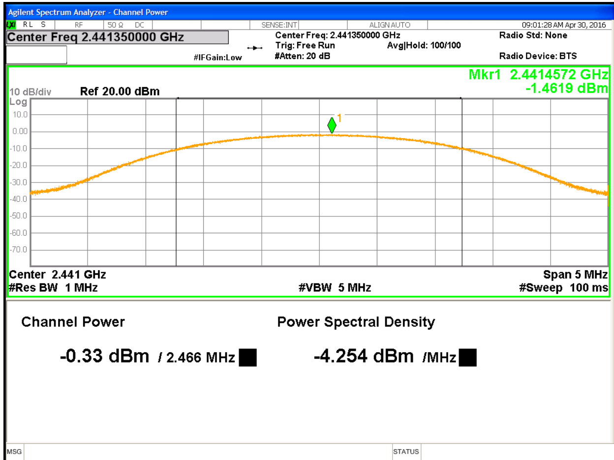
Figure 2: Maximum Conducted Output Power at 2441.35 MHz - Transmitter
