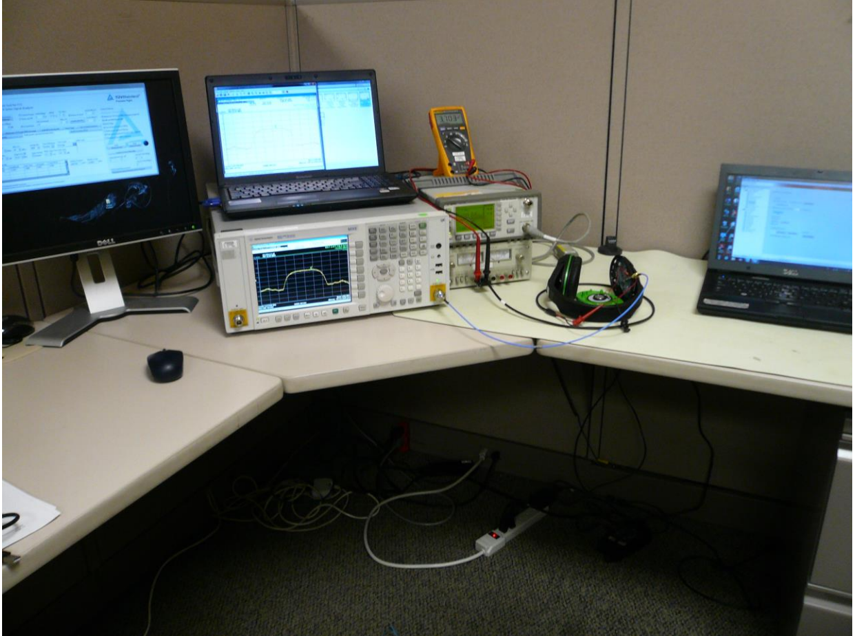
Figure 9: RF Conducted Test Setup
