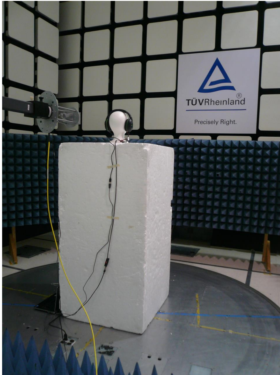
Figure 6: Test Setup for 18 GHz to 26 GHz (Rear View) - Y-Axis
