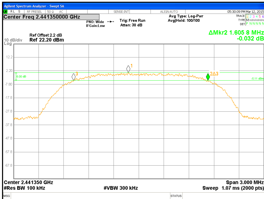
Figure 5: DTS Bandwidth-Headset -2441.35MHz
