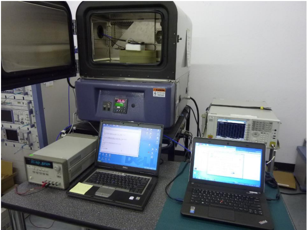
Figure 9: Frequency Stability Test Setup (Outside Thermo Chamber)
