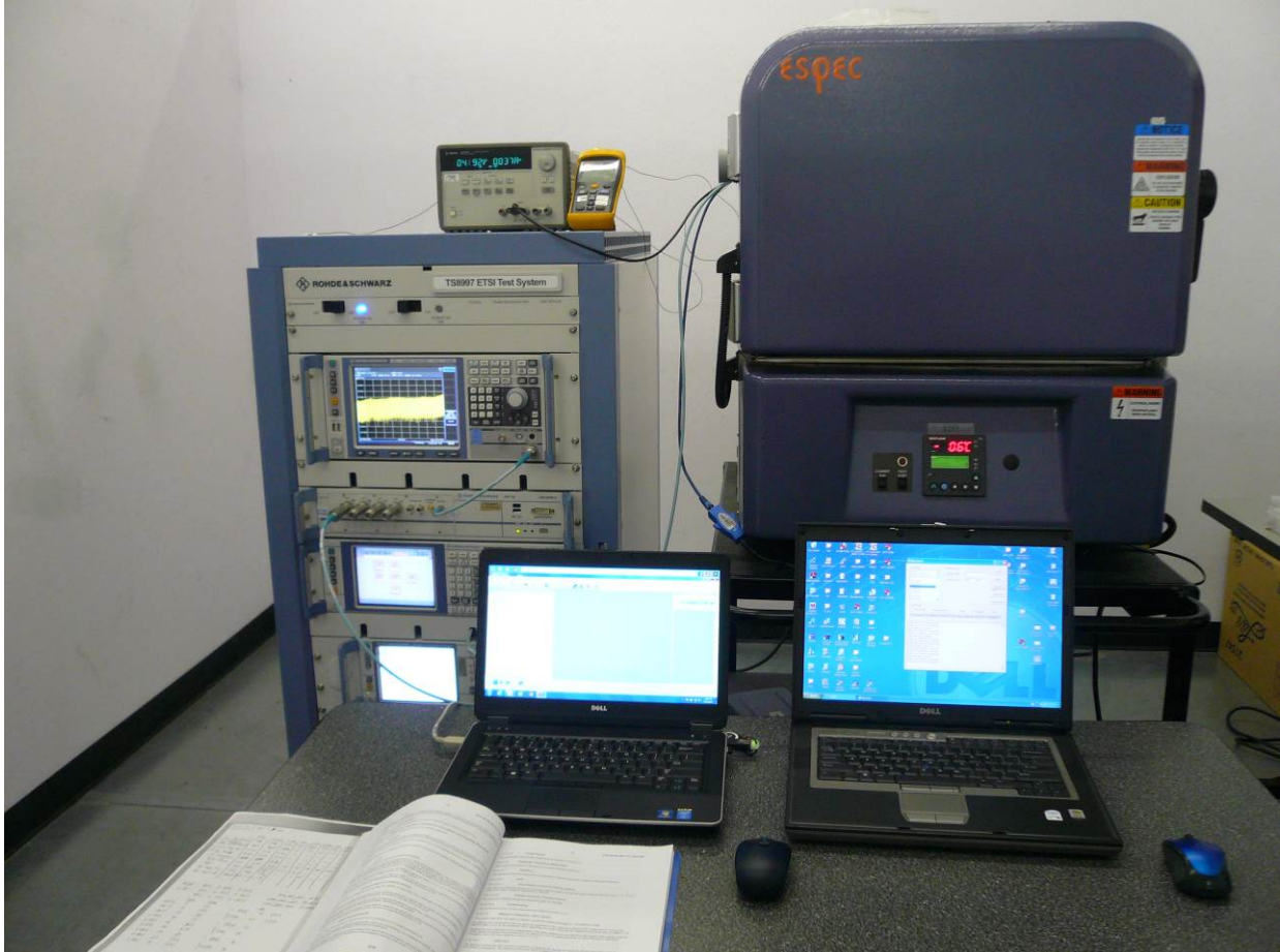
Figure 11: Frequency Stability Test Setup (Outside Thermo Chamber)
