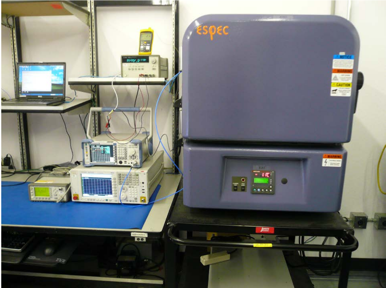
Figure 11: Frequency Stability Test Setup (Outside Thermo Chamber)
