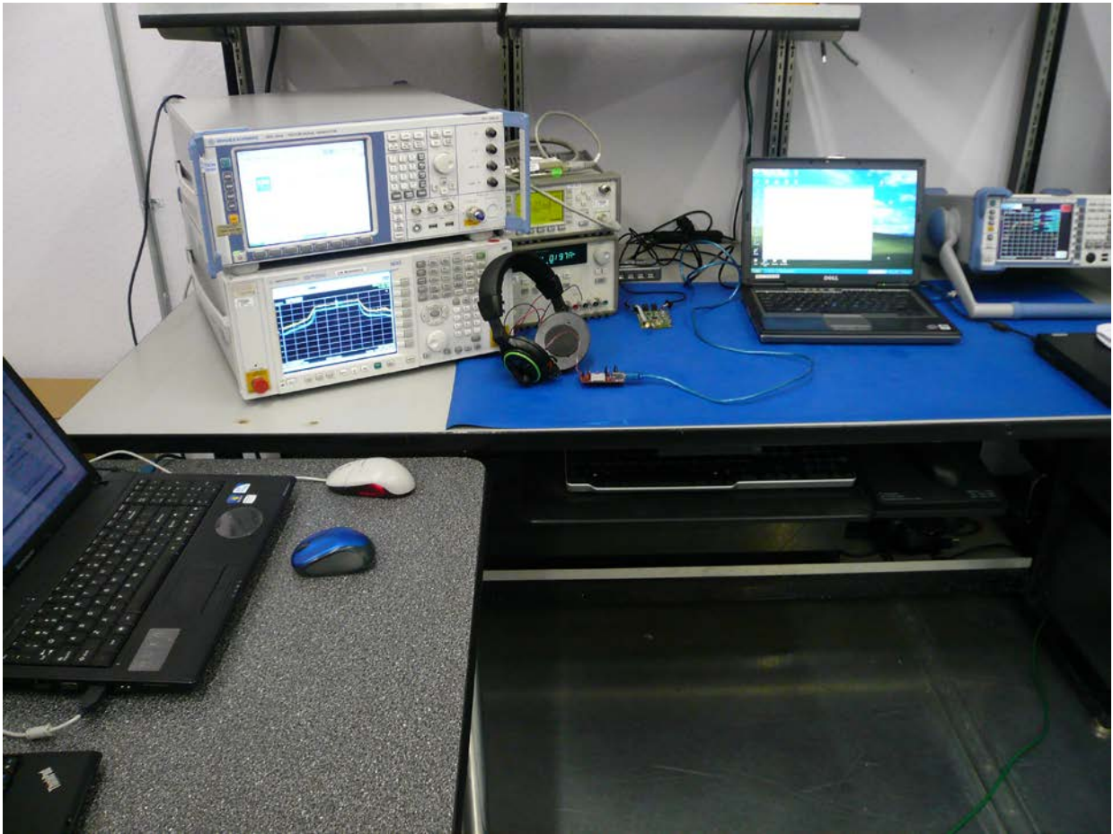
Figure 9: RF Conducted Test Setup
