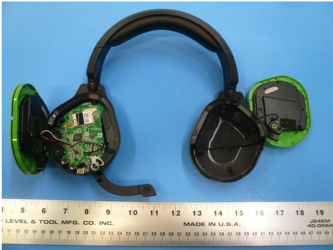
Figure 2: Internal Photo of Stealth 600X Gen 2 - Remove Speakers, Black version shown
