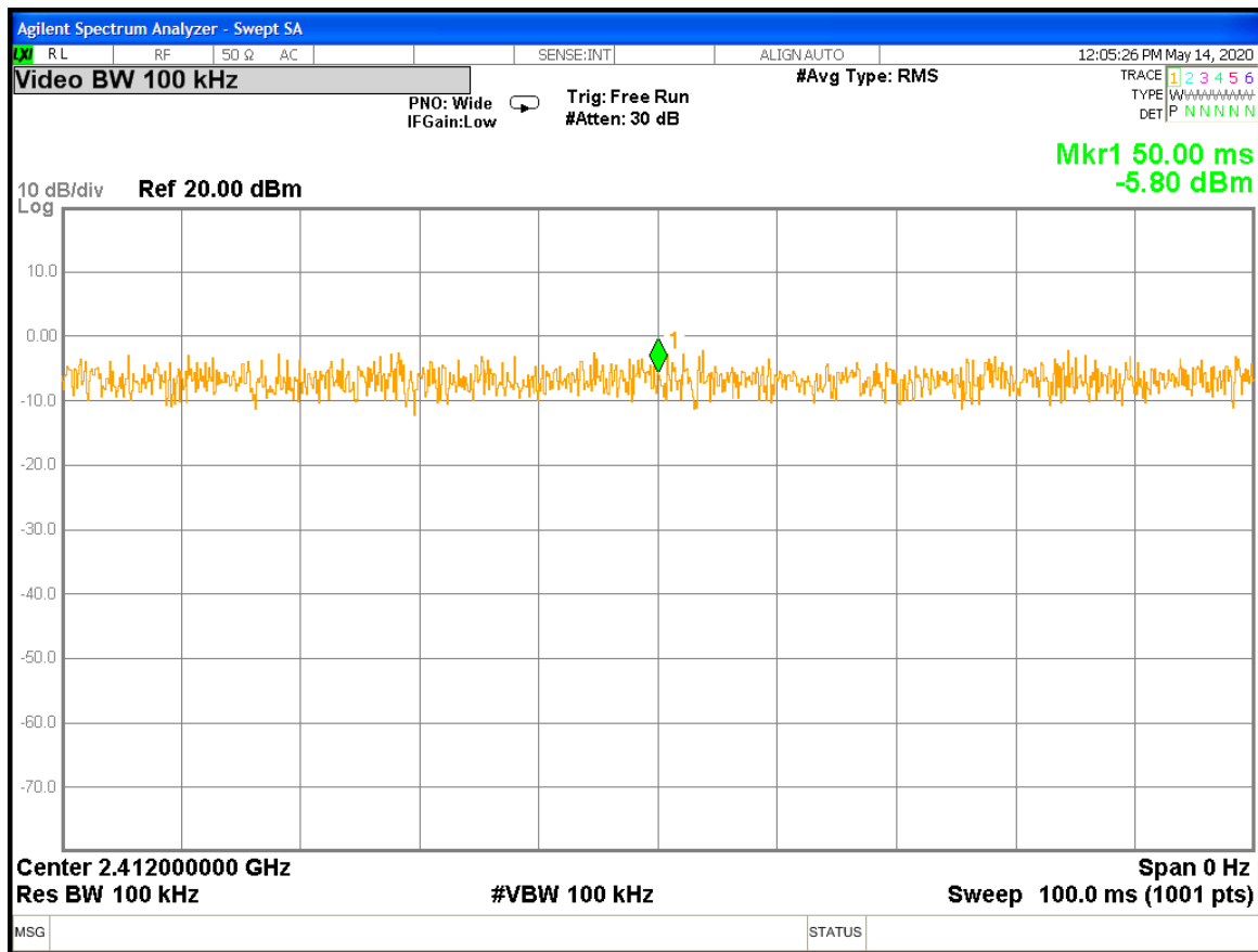
Figure 1: Duty Cycle for 802.11b
