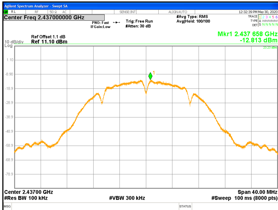
Figure 32: Maximum Power Spectral Density-2437 MHz-802.11b-1 Mbps
