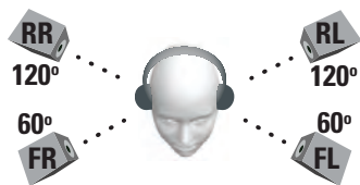
④ Front Angle; 60 degrees Rear Angle; 120 degrees
