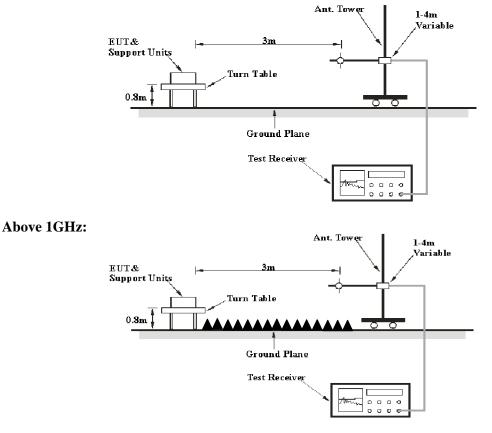
The radiated emission tests were performed in the 3 meters, using the setup accordance with the ANSI C63.4-2009. The specification used was the FCC 15.209, and FCC 15.407 limits.
