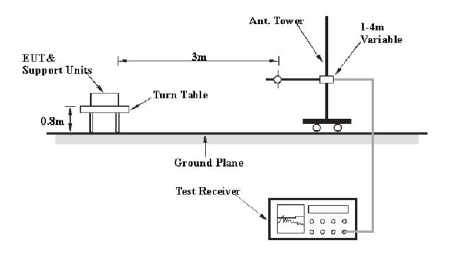
The radiated emission tests were performed in the 3 meters, using the setup accordance with the ANSI C63.4-2009. The specification used was the FCC 15.209, and FCC 15.407 limits.
