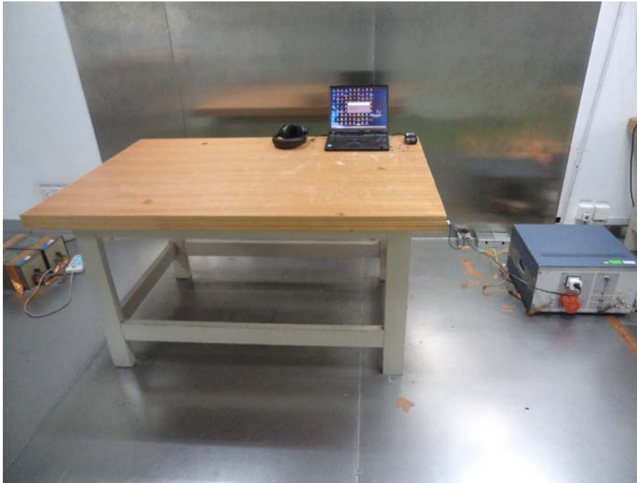
Conducted Emissions –Front View
