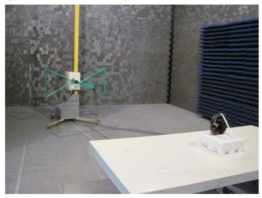
Description: Radiated Emission Test Setup for Below 1GHz-Mode 2
