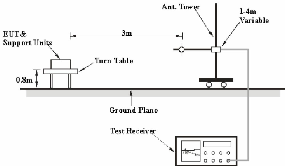
The radiated emission and out of band emission tests were performed in the 3 meters chamber B, using the setup accordance with the ANSI C63.4-2003. The specification used was the FCC 15.209, FCC 15.209 and FCC 15.249 limits.
