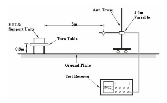
The radiated emission and out of band emission tests were performed in the 3 meters chamber B, using the setup accordance with the ANSI C63.4-2003. The specification used was the FCC 15.209, FCC 15.109 and FCC 15.249 limits.
