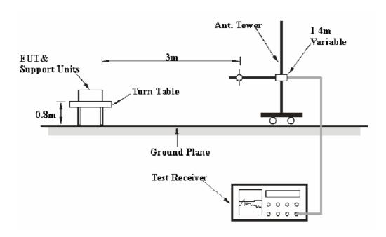
The radiated emission and out of band emission tests were performed in the 3 meters chamber B, using the setup accordance with the ANSI C63.4-2003. The specification used was the FCC 15.209 and FCC 15.249 limits.
