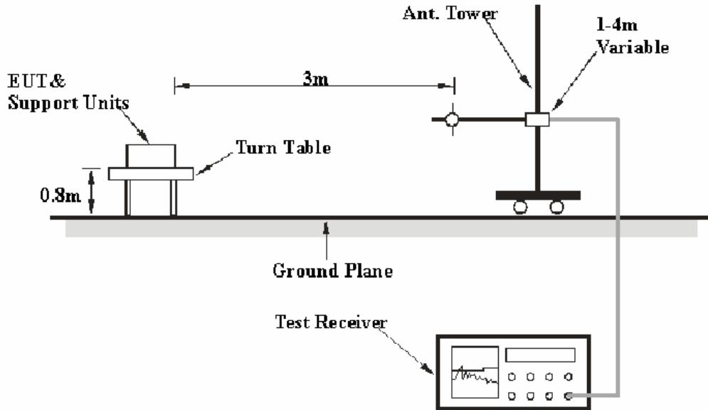
The radiated emission and out of band emission tests were performed in the 3 meters chamber B, using the setup accordance with the ANSI C63.4-2003. The specification used was the FCC 15.209, FCC 15.109 and FCC 15.249 limits.
