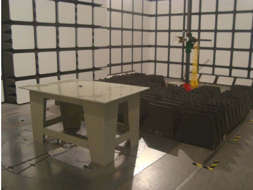
Radiated Emissions - Rear View (Above 1 GHz)
