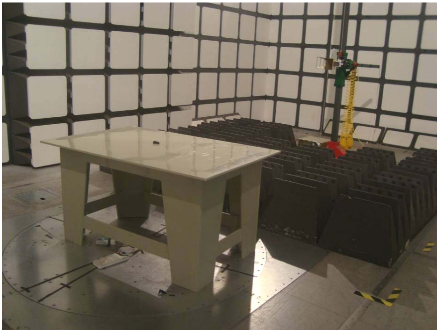
Radiated Emissions - Rear View (Above 1 GHz)
