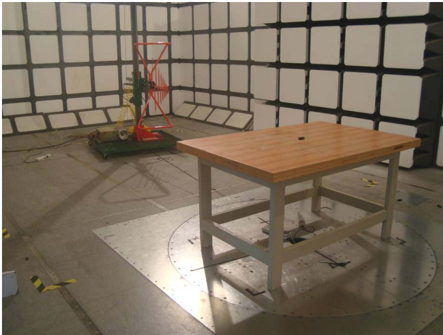
Radiated Emissions - Rear View (Below 1 GHz)
