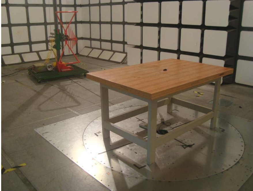
Radiated Emissions - Rear View (Below 1 GHz)
