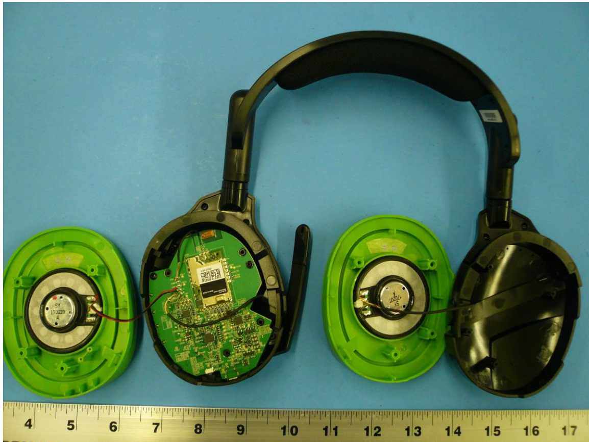
Figure 2: Internal Photo of Ear Force Stealth 600X - Remove Speakers
