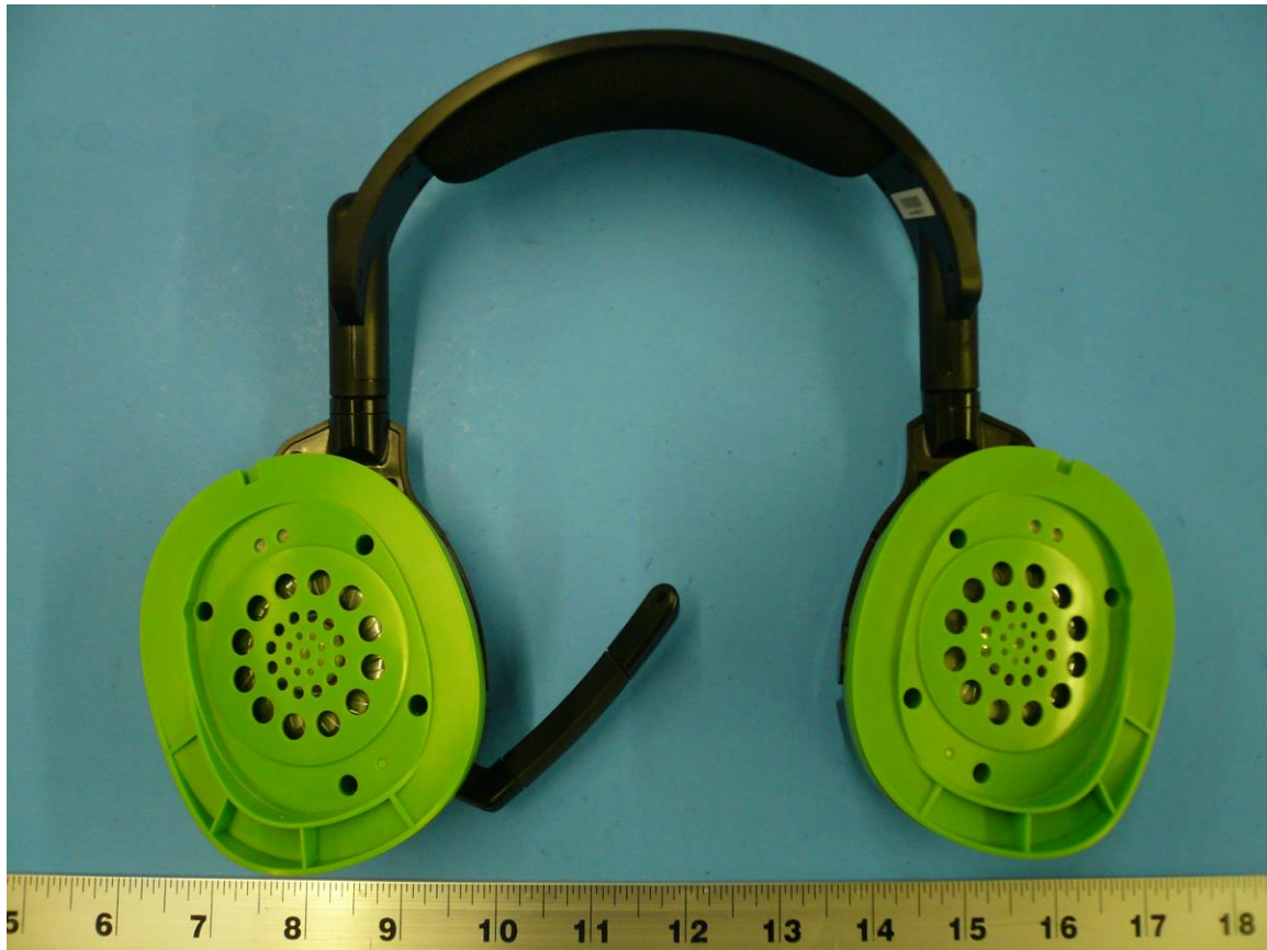
Figure 1: Internal Photo of Ear Force Stealth 600X without Ear Cover
