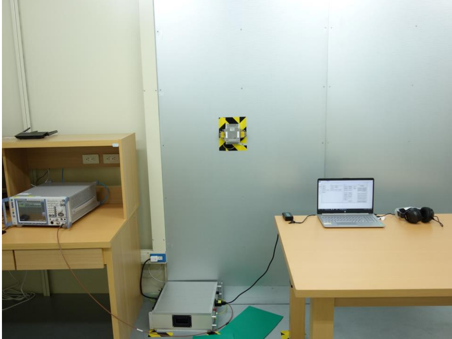
Photograph 7: Set-up for AC Mains (Front View)
