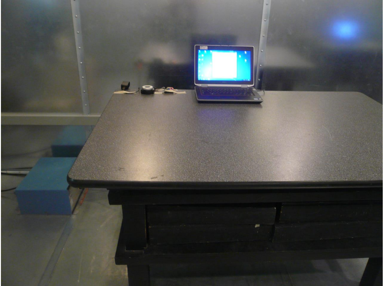
Figure 9: AC Conducted Emission Test Setup (Front)
