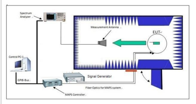
Figure 1. 2D antenna pattern test system.
