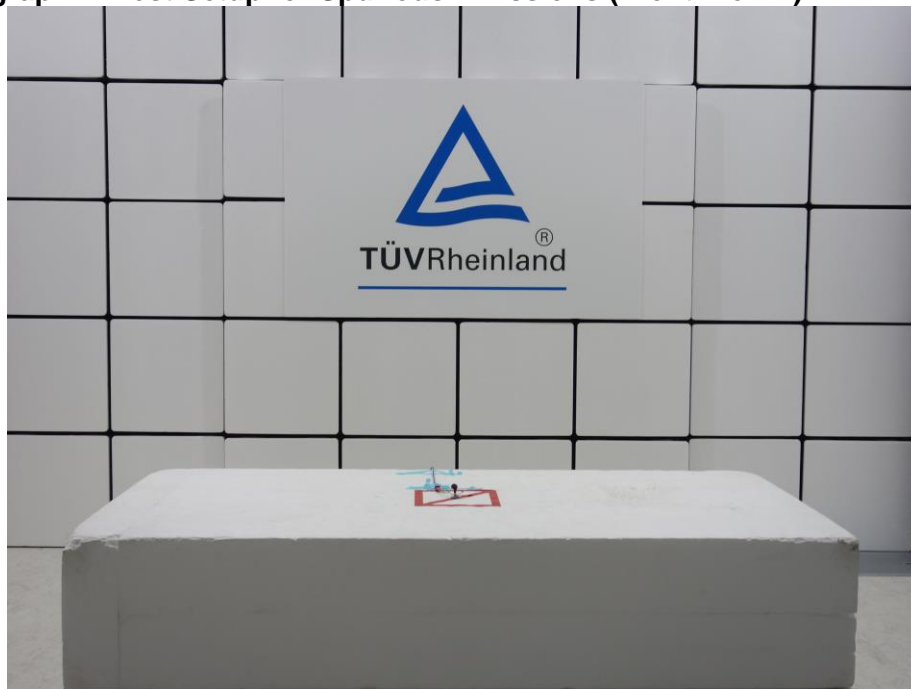
Photograph 2: Test Setup for Spurious Emissions (Front View 2)
