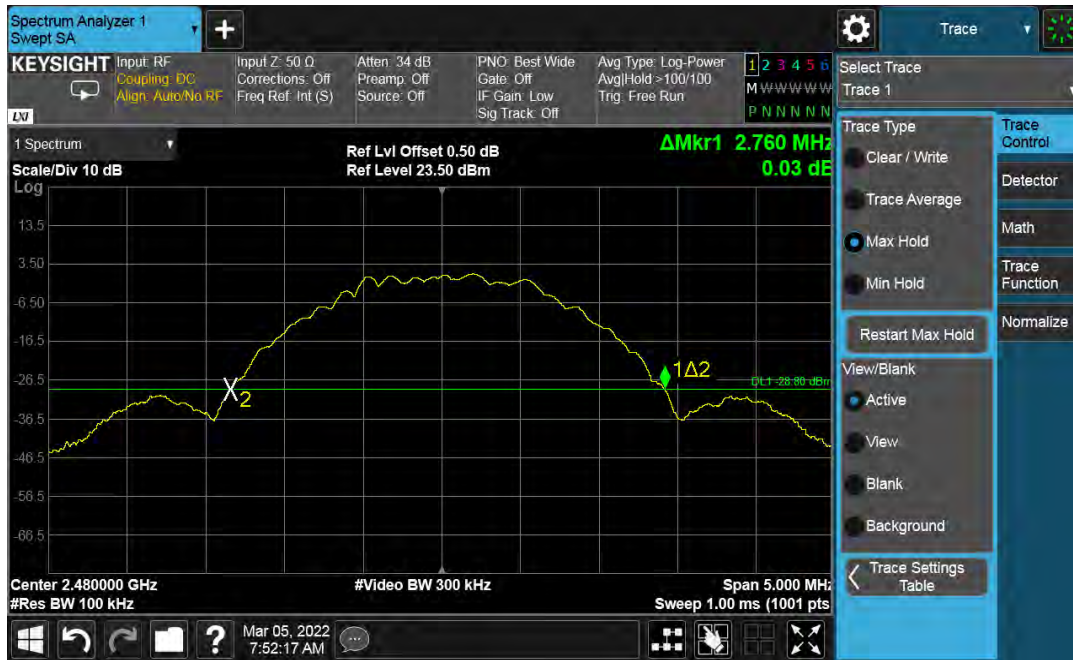
Figure 36: Conducted Band Edge - 2480 MHz at 2 Mbps
