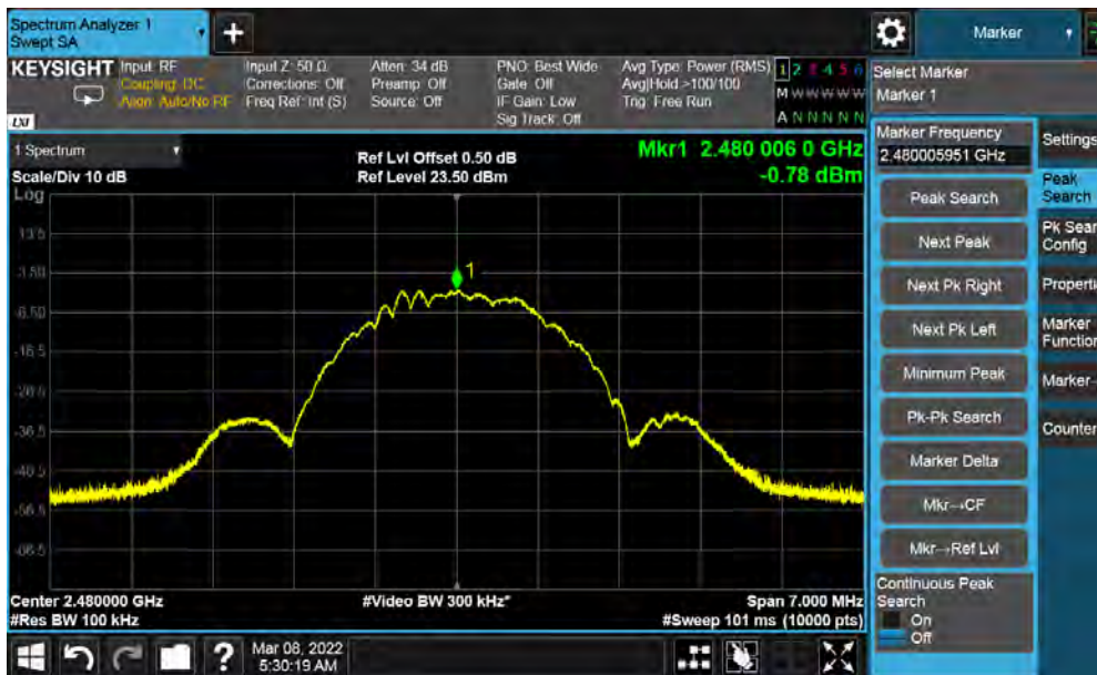
Figure 25: Maximum Power Spectral Density-2480 MHz at 2 Mbps
