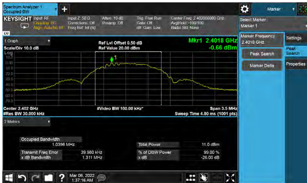
Figure 11: 99% Bandwidth 2402 MHz at 1Mbps
