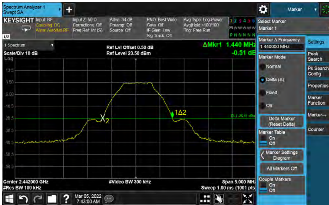
Figure 28: Conducted Band Edge - 2442 MHz at 1 Mbps
