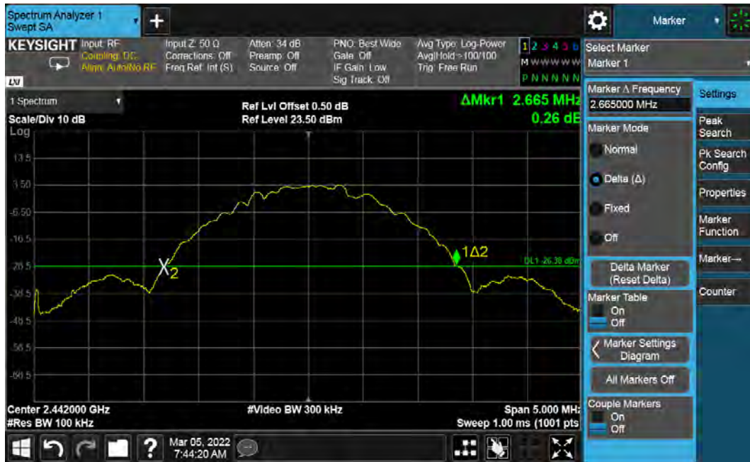
Figure 34: Conducted Band Edge - 2442 MHz at 2 Mbps
