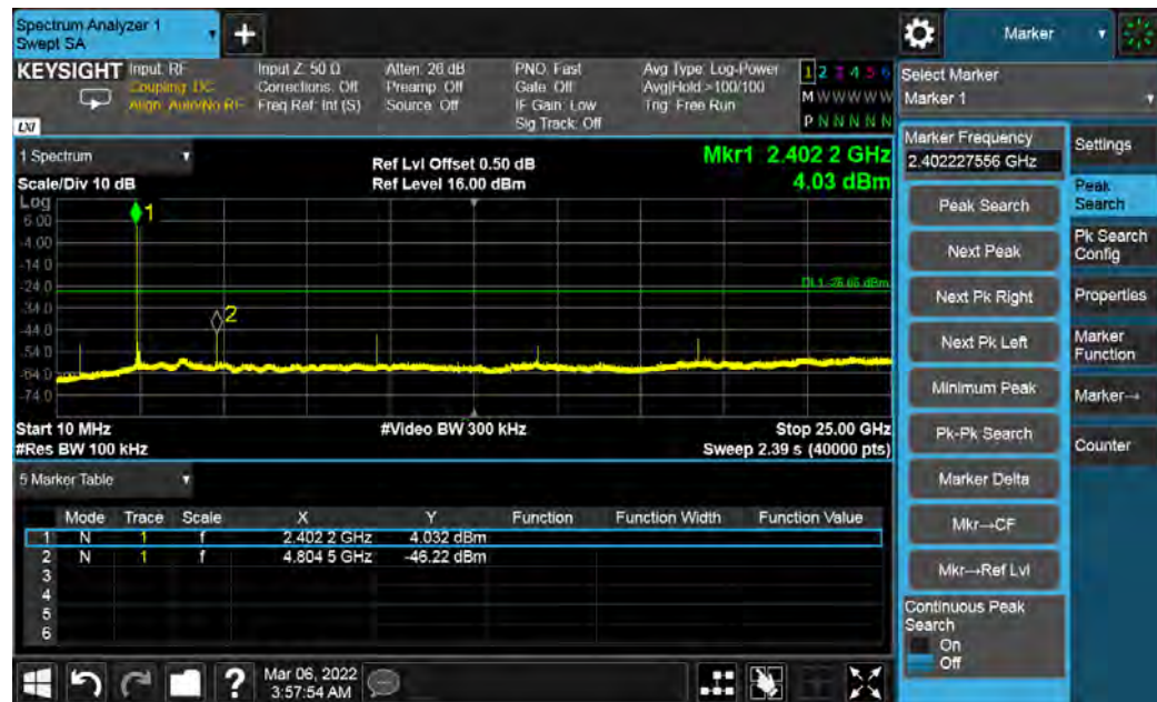
Figure 27: Out of band Emission - 2402 MHz at 1 Mbps
