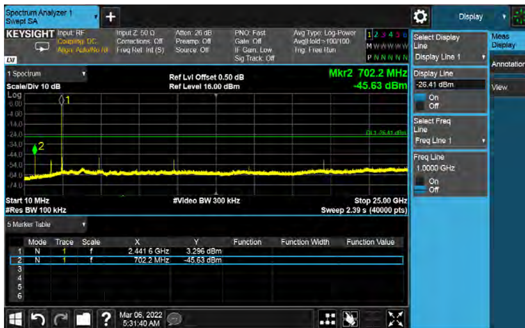
Figure 29: Out of band Emission - 2442 MHz at 1 Mbps
