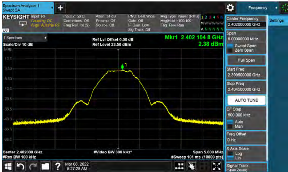
Figure 20: Maximum Power Spectral Density-2402 MHz at 1 Mbps
