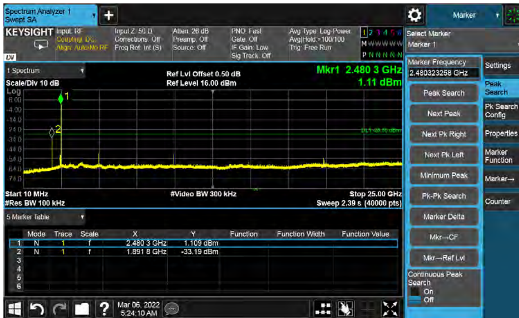
Figure 37: Out of band Emission - 2480 MHz at 2 Mbps
