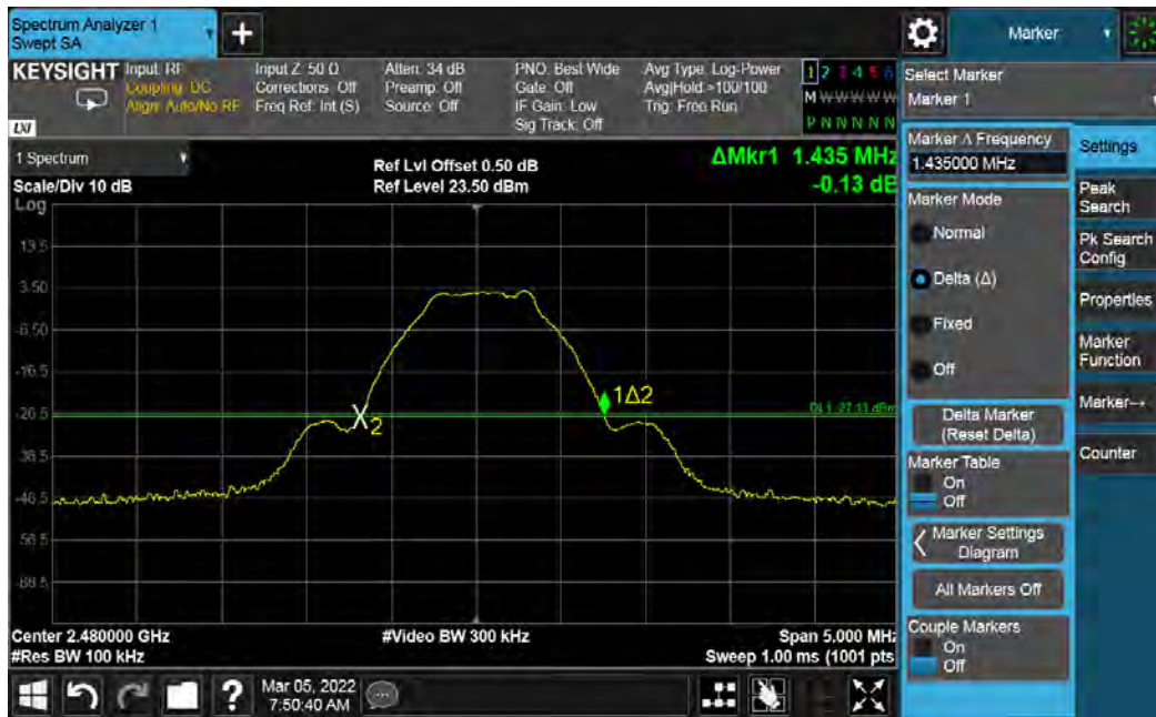
Figure 30: Conducted Band Edge - 2480 MHz at 1 Mbps
