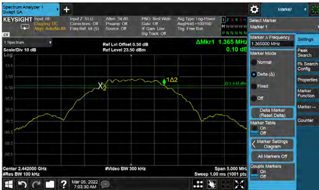
Figure 15: DTS Bandwidth 2442 MHz at 2 Mbps
