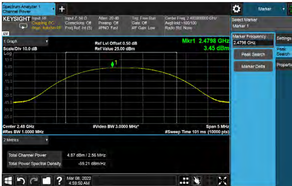
Figure 4: Maximum Conducted Output Power at 2480 MHz at 1Mbps
