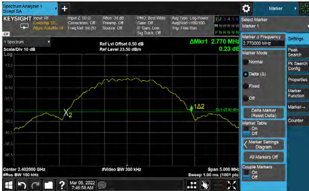
Figure 32: Conducted Band Edge - 2402 MHz at 2 Mbps
