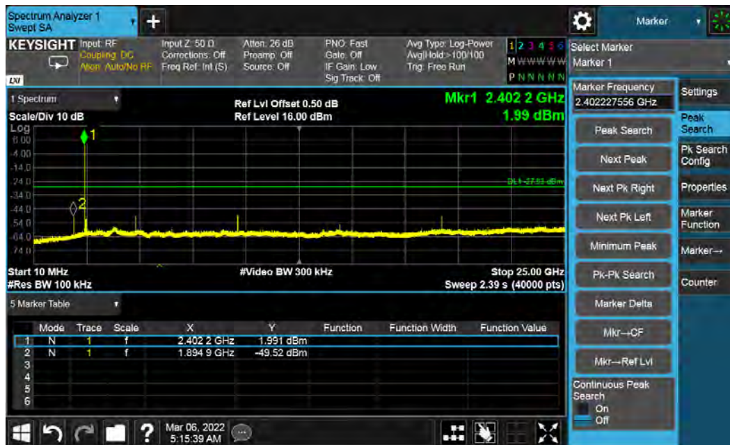
Figure 33: Out of band Emission - 2402 MHz at 2 Mbps
