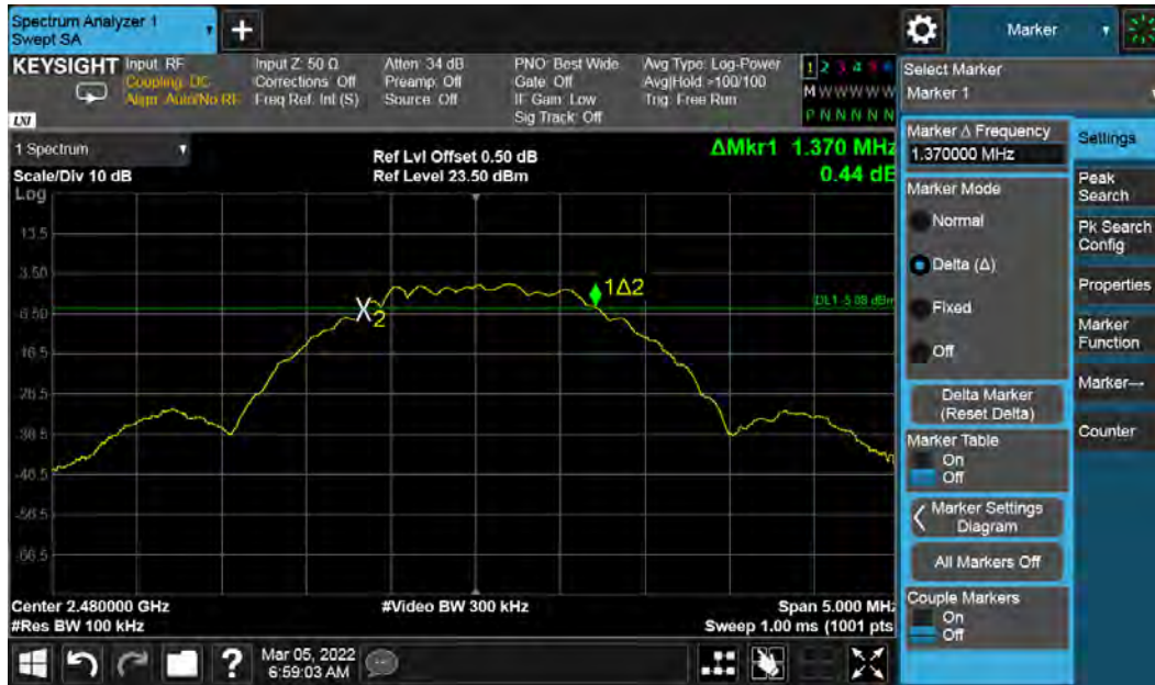
Figure 16: DTS Bandwidth 2480 MHz at 2 Mbps
