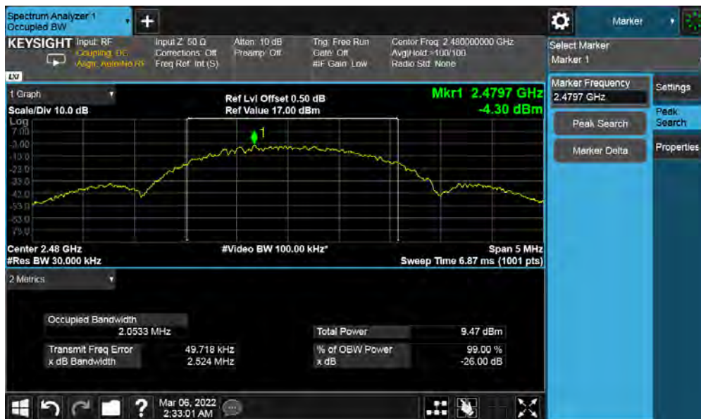
Figure 19: 99% Bandwidth 2480 MHz at 2 Mbps
