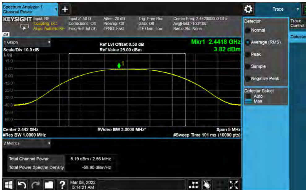
Figure 3: Maximum Conducted Output Power at 2442 MHz at 1Mbps
