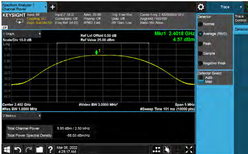
Figure 2: Maximum Transmitted Power, 2402 MHz at 1Mbps
