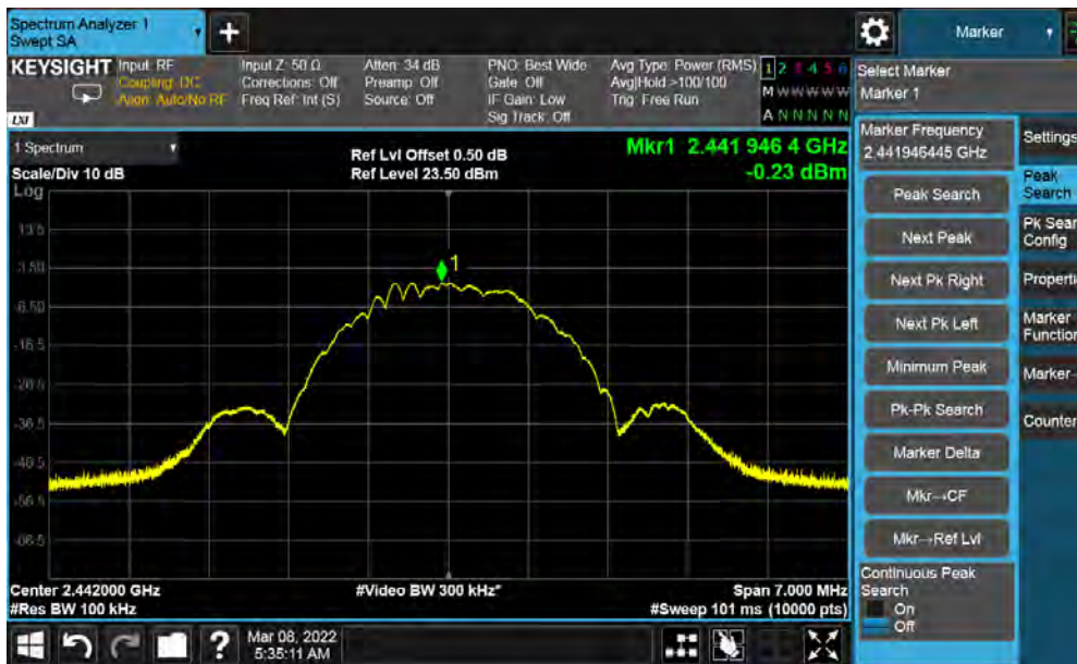
Figure 24: Maximum Power Spectral Density-2442 MHz at 2 Mbps
