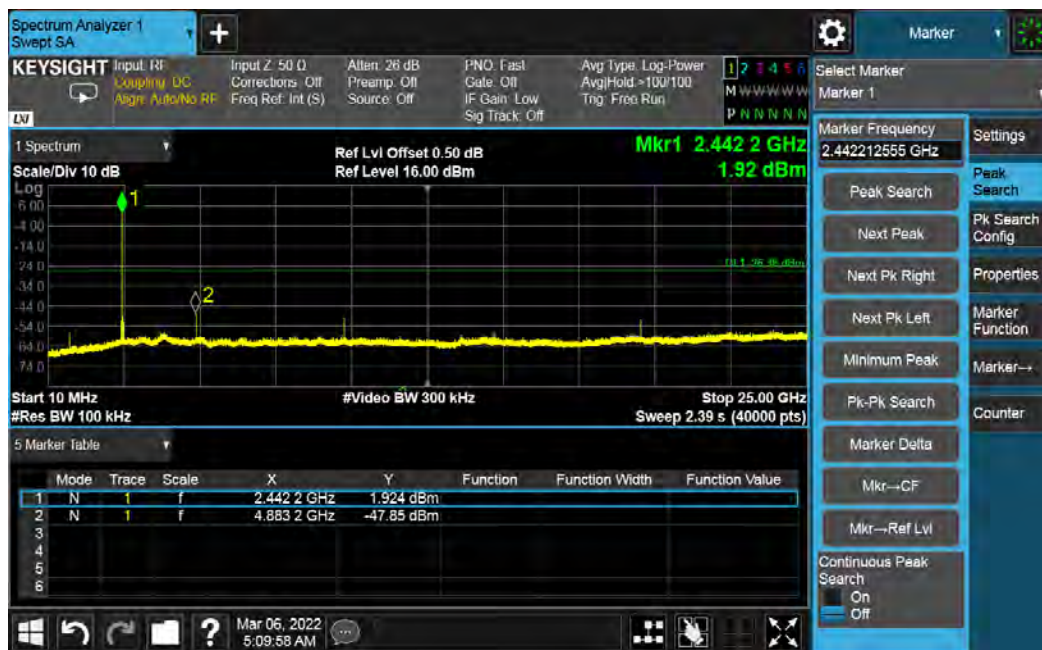
Figure 35: Out of band Emission - 2442 MHz at 2 Mbps
