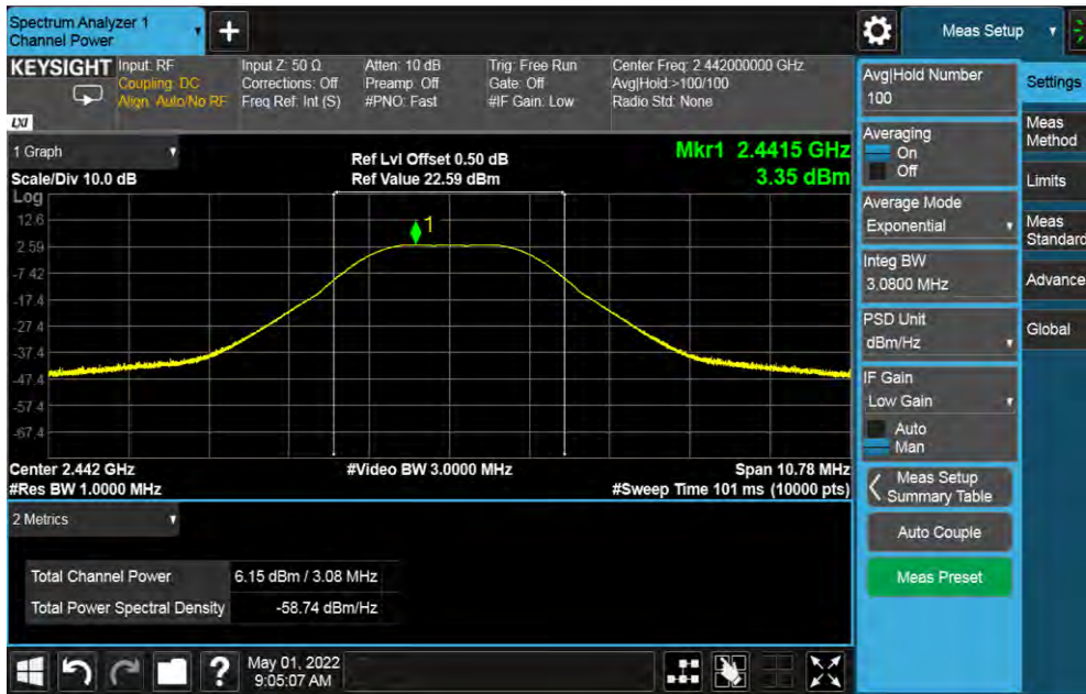
Figure 6: Maximum Conducted Output Power at 2442 MHz at 2Mbps
