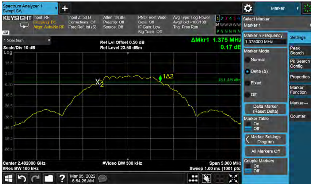
Figure 14: DTS Bandwidth 2402 MHz at 2 Mbps
