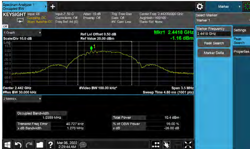
Figure 12: 99% Bandwidth 2442 MHz at 1Mbps
