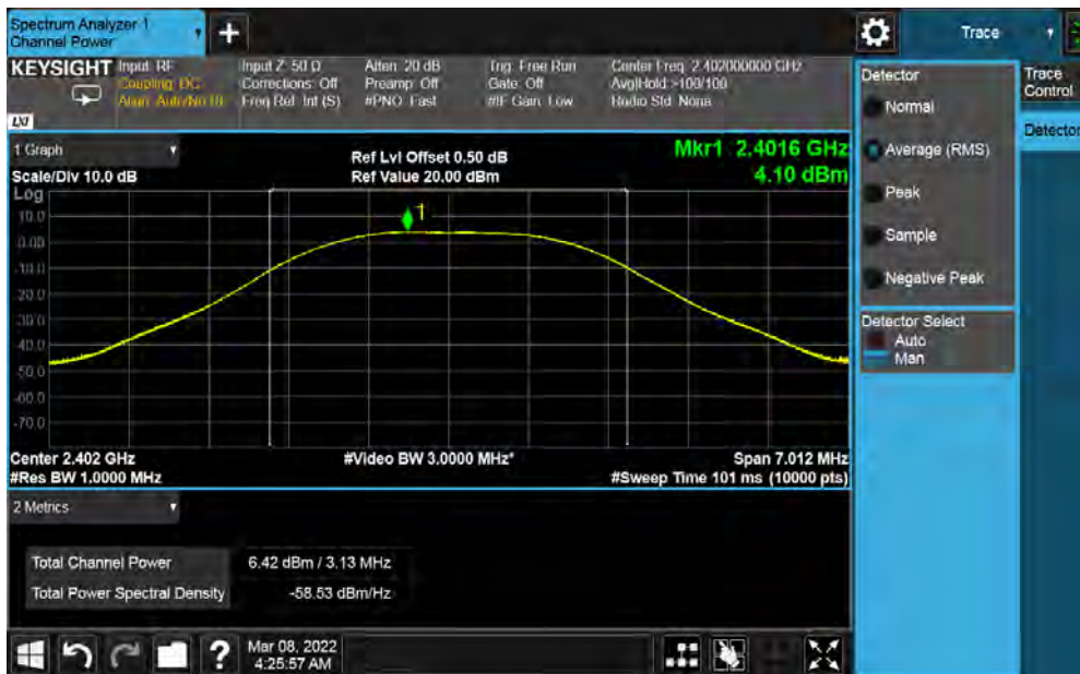
Figure 5: Maximum Conducted Output Power at 2402 MHz at 2Mbps
