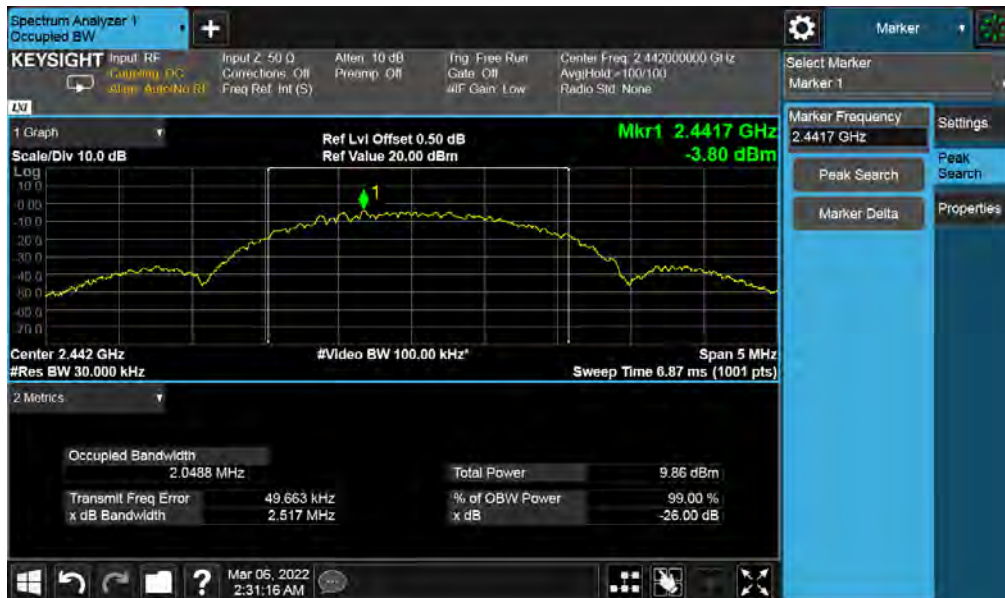
Figure 18: 99% Bandwidth 2442 MHz at 2 Mbps
