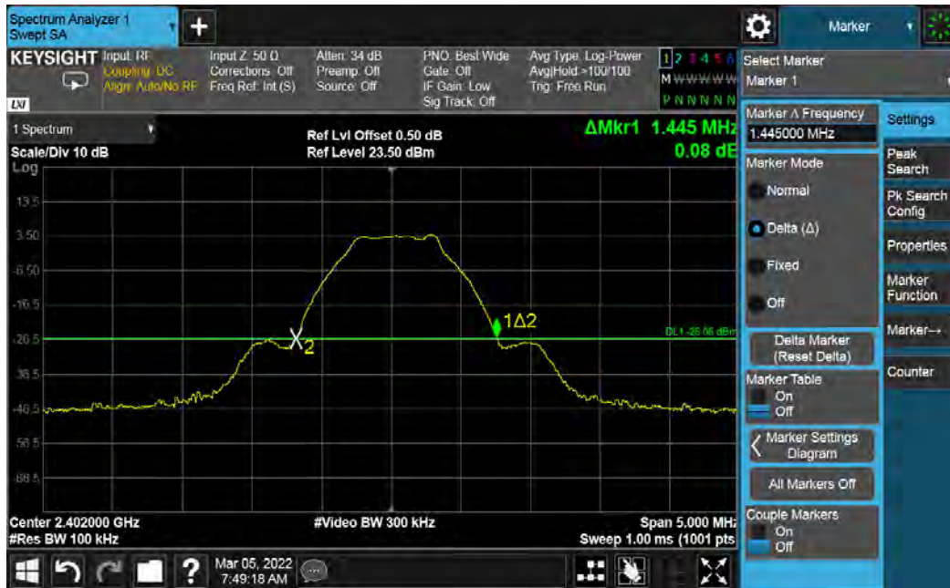
Figure 26: Conducted Band Edge - 2402 MHz at 1 Mbps
