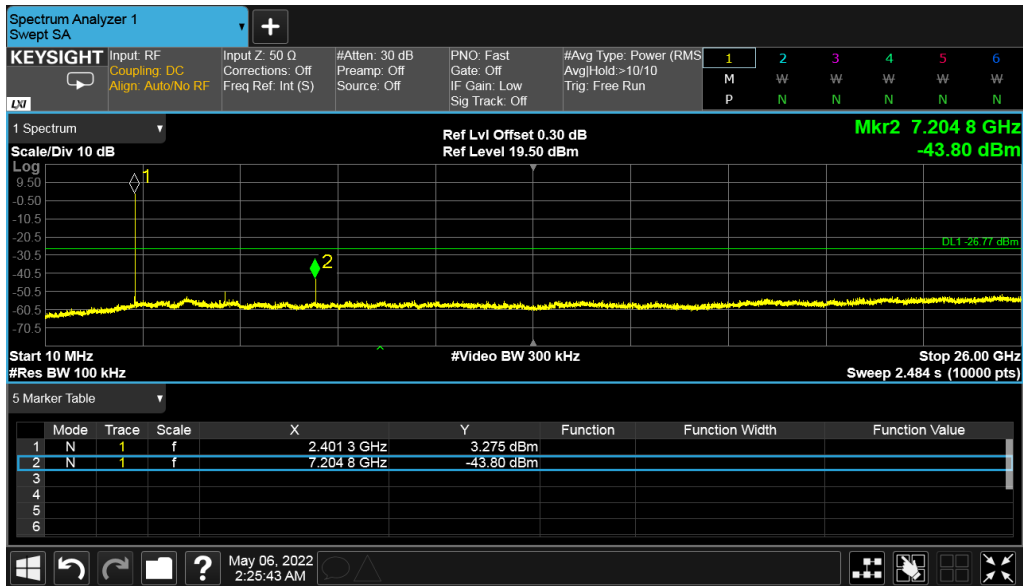
Figure 15: Out of band Emission - 2402 MHz at 1 Mbps
