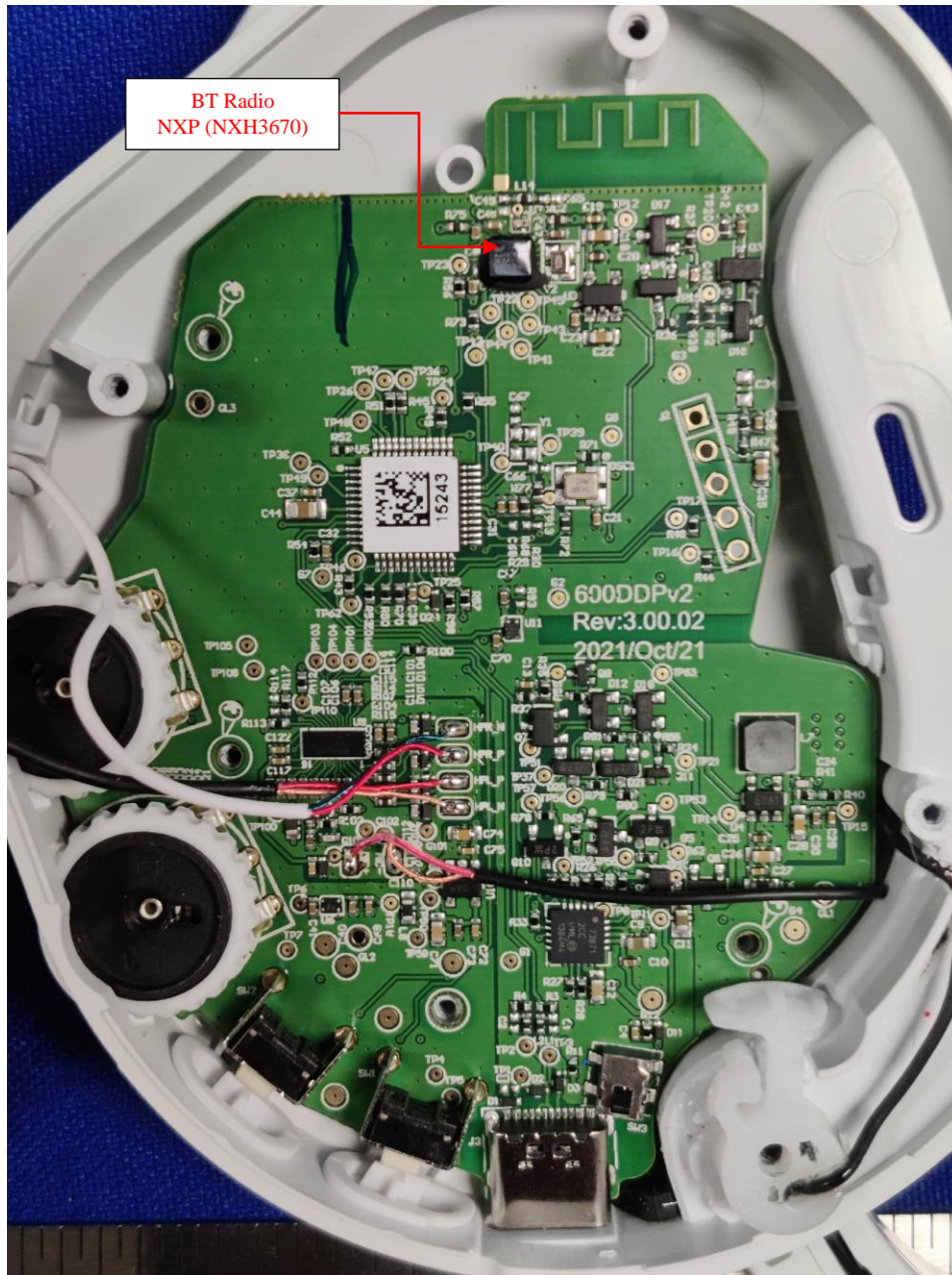
Figure 2: Internal Photo of Stealth600P-USB-RX – Top PCB
