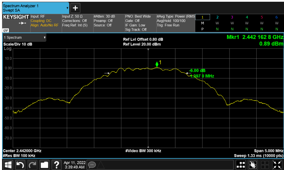
Figure 16: DTS Bandwidth 2442 MHz at 2 Mbps
