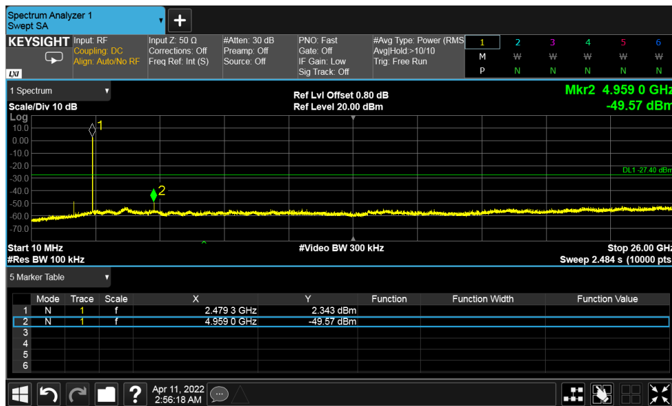
Figure 32: Out of band Emission - 2480 MHz at 1 Mbps
