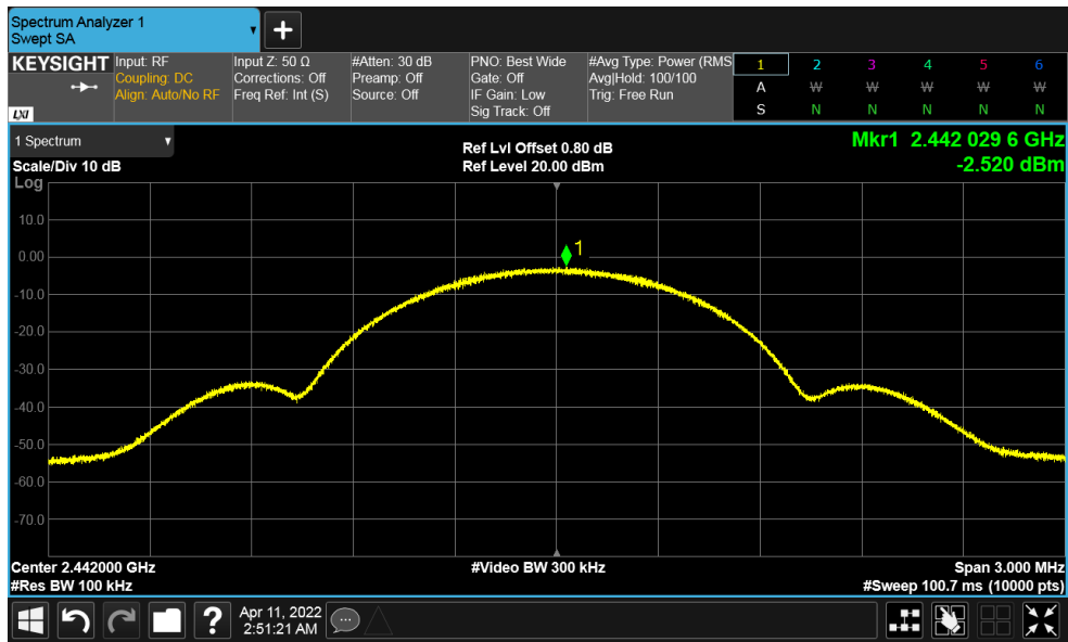
Figure 22: Maximum Power Spectral Density-2442 MHz at 1 Mbps
