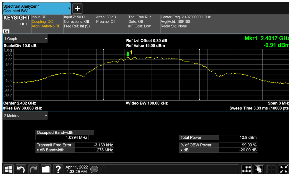
Figure 12: 99% Bandwidth 2402 MHz at 1Mbps
