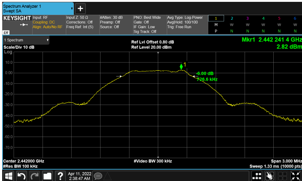
Figure 10: DTS Bandwidth 2442 MHz at 1 Mbps
