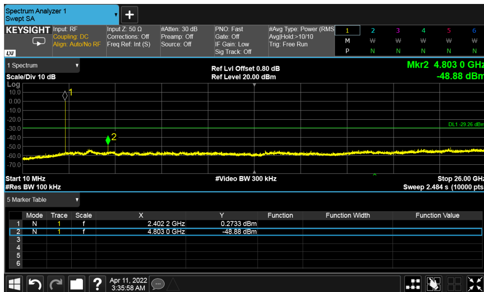
Figure 34: Out of band Emission - 2402 MHz at 2 Mbps
