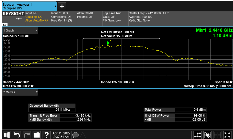
Figure 13: 99% Bandwidth 2442 MHz at 1Mbps
