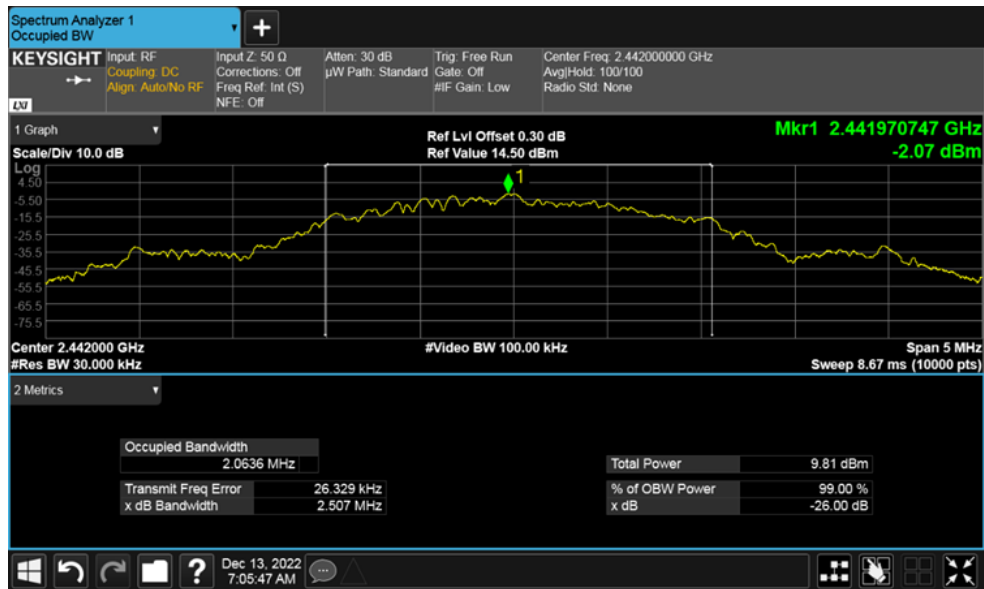
Figure 9: 99% Bandwidth 2442 MHz at 2 Mbps
