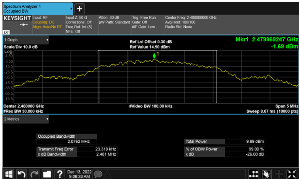
Figure 10: 99% Bandwidth 2480 MHz at 2 Mbps
