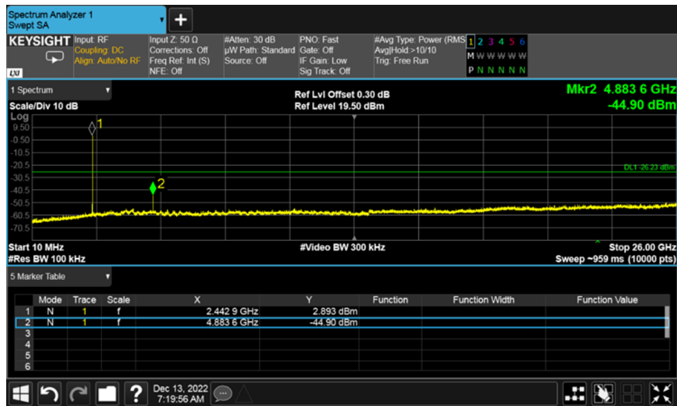
Figure 17: Out of band Emission - 2442 MHz at 2 Mbps
