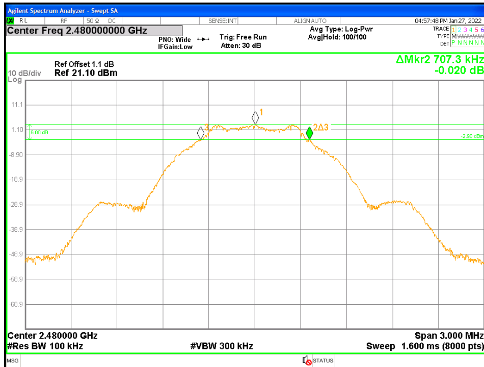
Figure 11: DTS Bandwidth - Transmitter at 1 Mbps - 2480 MHz
