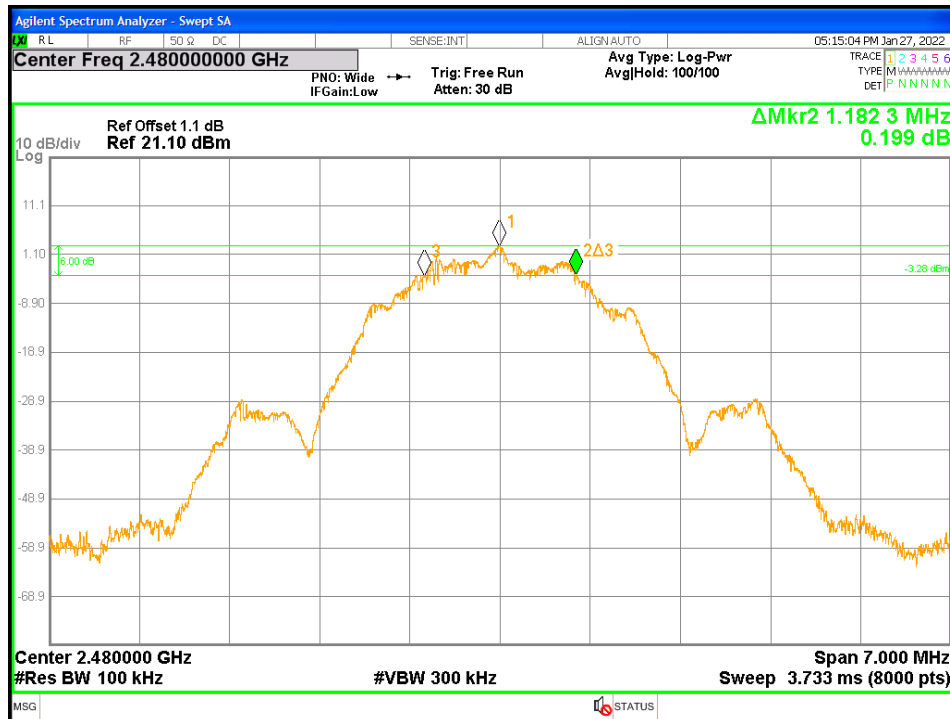
Figure 17: DTS Bandwidth - Transmitter at 2 Mbps - 2480 MHz
