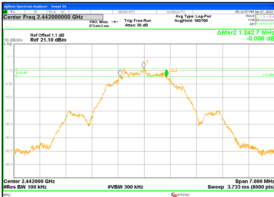
Figure 16: DTS Bandwidth - Transmitter at 2 Mbps - 2442 MHz
