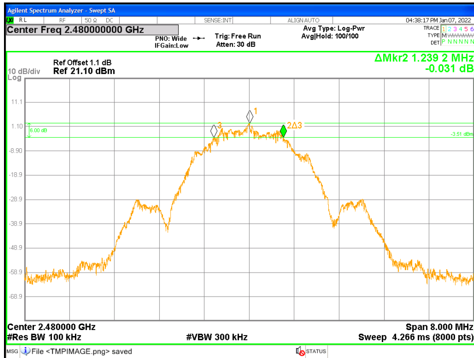
Figure 17: DTS Bandwidth-Headset at 2Mbps - 2480 MHz
