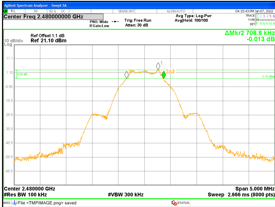
Figure 11: DTS Bandwidth-Headset at 1Mbps - 2480 MHz
