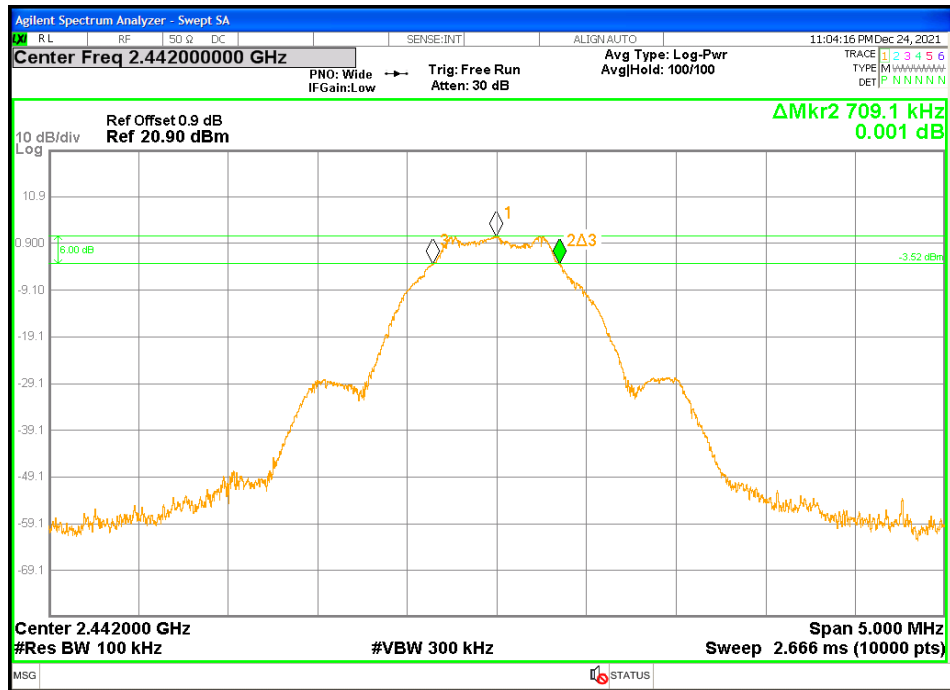
Figure 10: DTS Bandwidth - Transmitter at 1 Mbps - 2442 MHz
