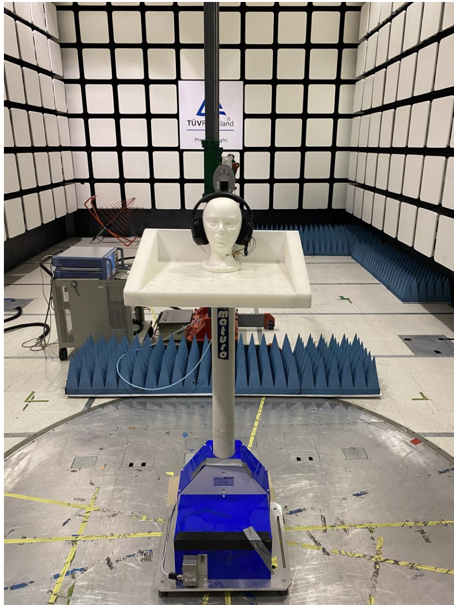
Figure 7: Test Setup for 18 GHz to 26 GHz (Front View)
