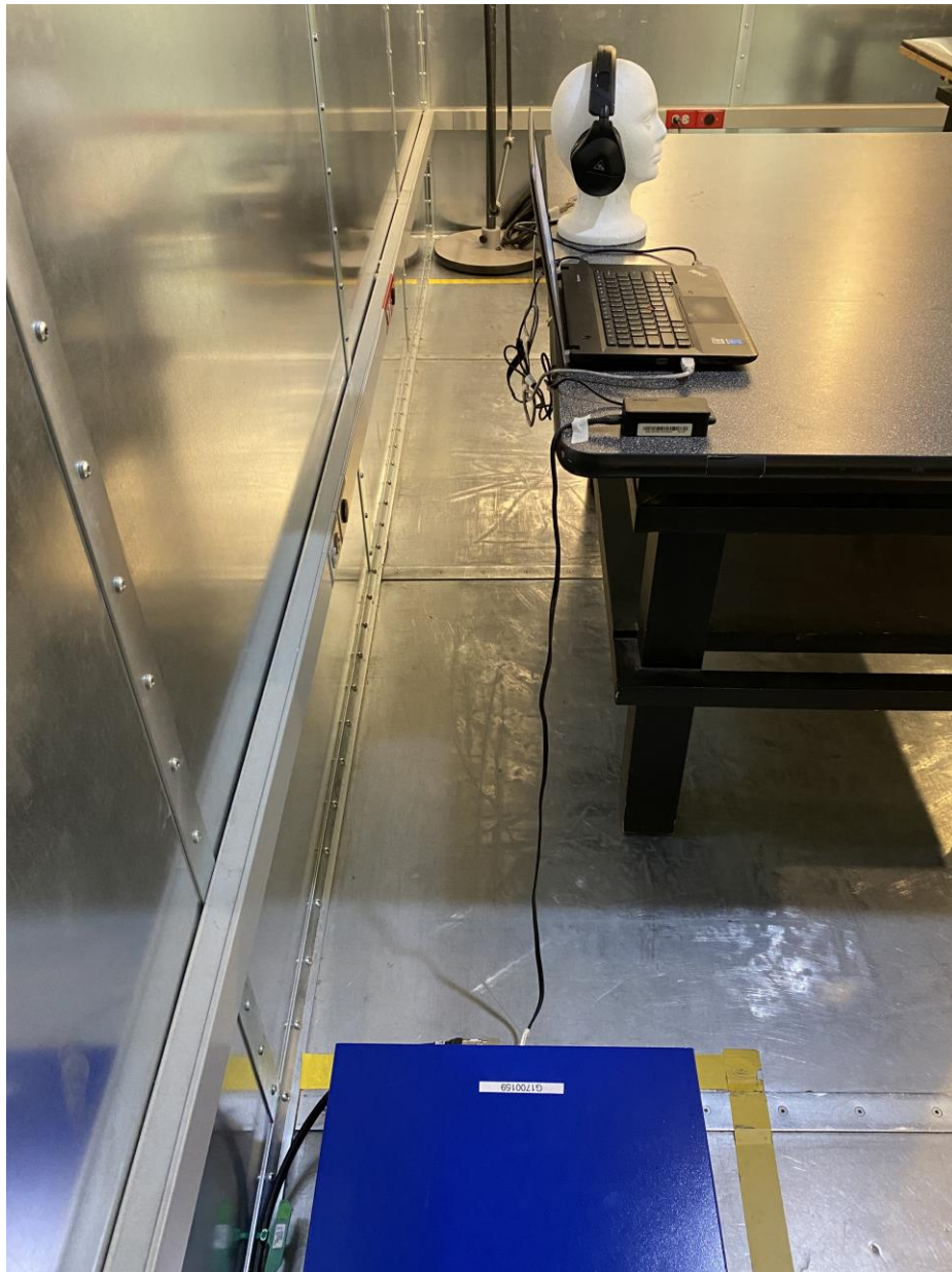
Figure 11: AC Conducted Emission Test Setup (Side View)
