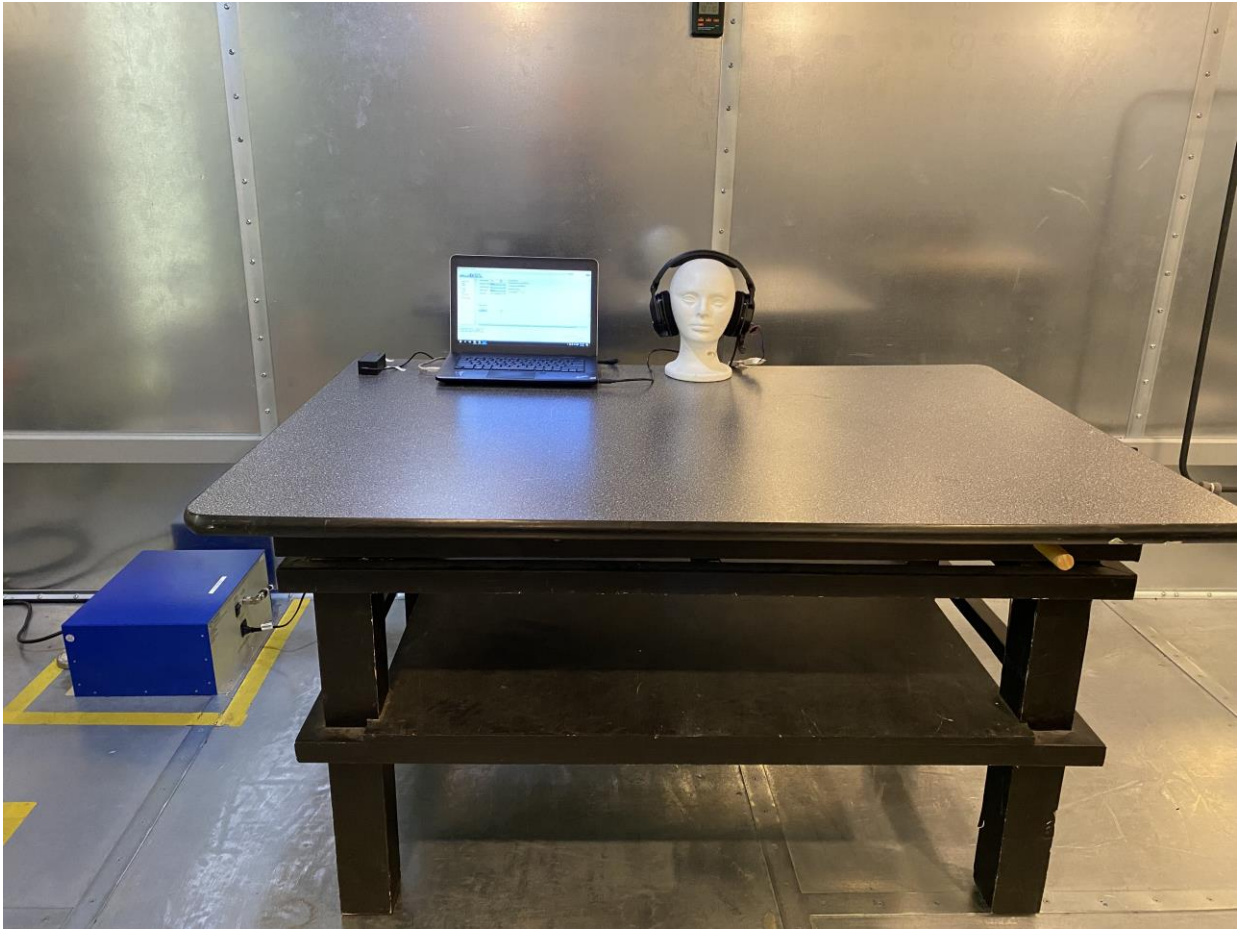
Figure 10: AC Conducted Emission Test Setup (Front View)
