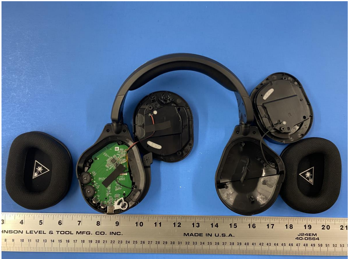
Figure 1: Internal Photo of Stealth 600X Gen 2 MAX RX - Remove Speakers
