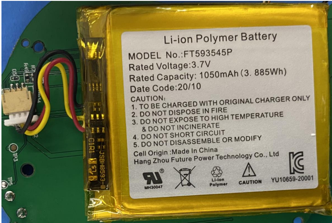
Figure 5: Internal Photo of Stealth 600X Gen 2 MAX RX (1050 mAh Battery, Top)
