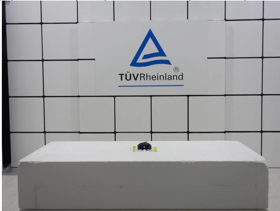
Photograph 2: Test Setup for Spurious Emissions (Front View 2)
