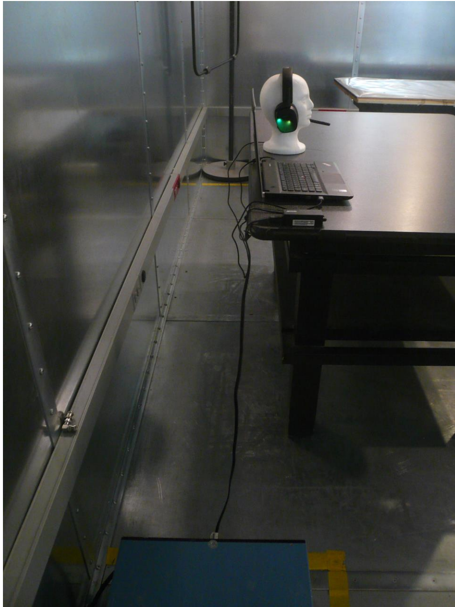
Figure 11: AC Conducted Emission Test Setup (Rear View)
