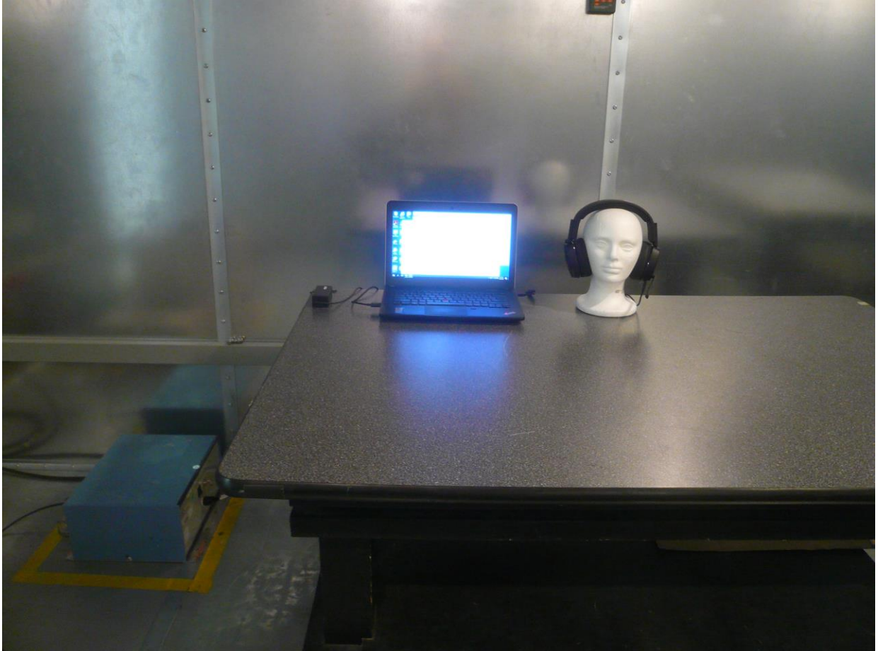
Figure 10: AC Conducted Emission Test Setup (Front View)
