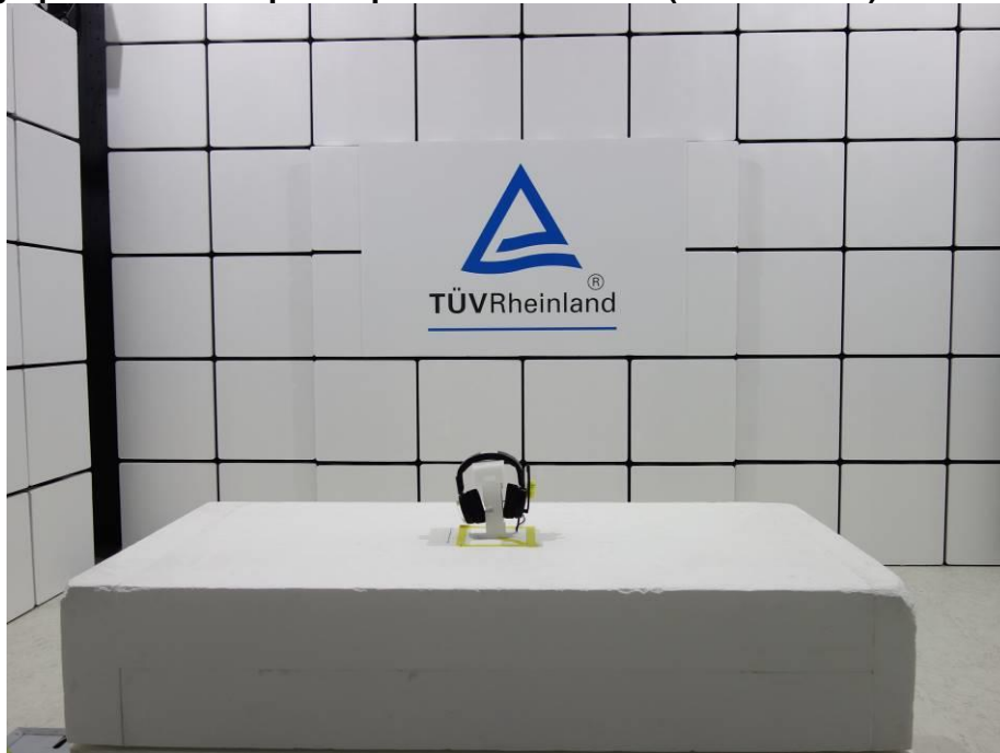
Photograph 2: Test Setup for Spurious Emissions (Front View 2)
