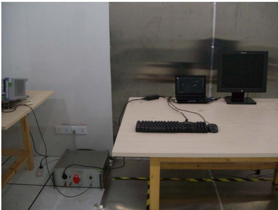
Line Conducted Emission Test Setup
