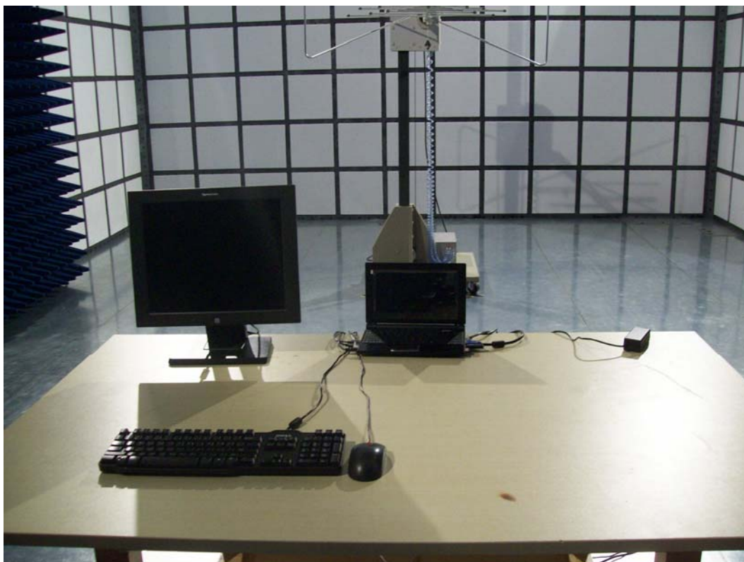
Radiated Emission Test Setup
