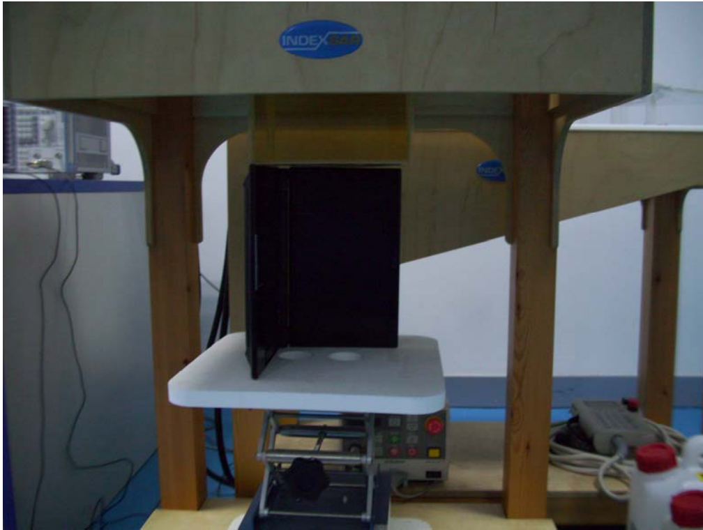
Fig.9 Side Position 1 (CDMA 2000 antenna against flat phantom)
