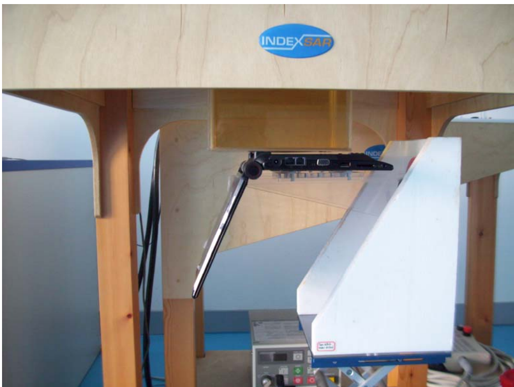
Fig.9 Side Position 2 (CDMA 2000 antenna against flat phantom)
