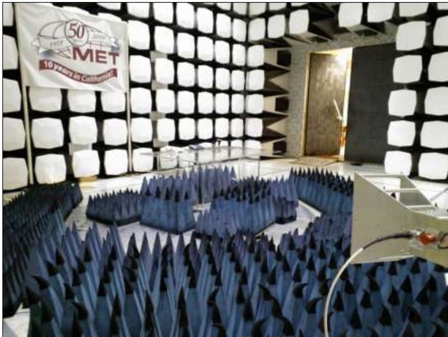
Photograph 6. Radiated Emission, Test Setup, 1 GHz – 6 GHz, Telo
