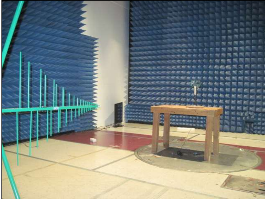
Photograph 9. Radiated Spurious Emissions, 30 MHz – 1 GHz
