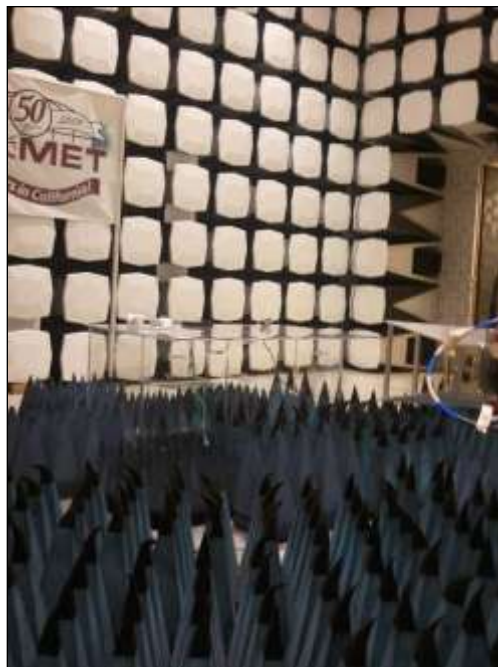
Photograph 4. Radiated Emission, Test Setup, 1 GHz – 6 GHz, Schmidt
