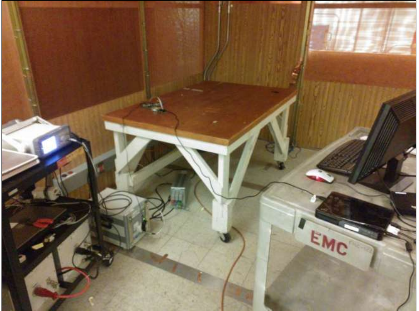
Photograph 8. Conducted Emissions, 15.207(a), Test Setup
