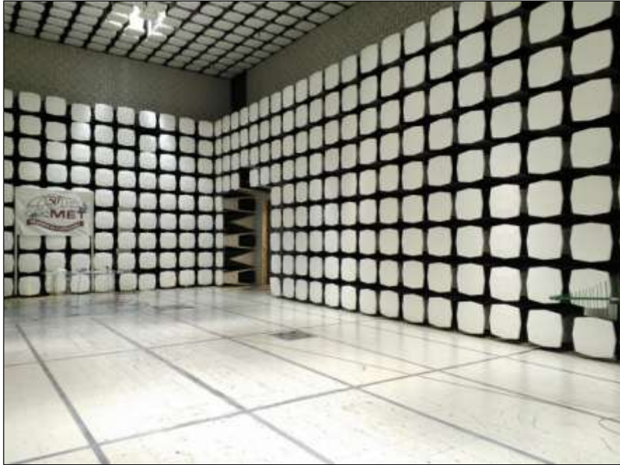
Photograph 5. Radiated Emission, Test Setup, 30 MHz – 1 GHz, Telo
