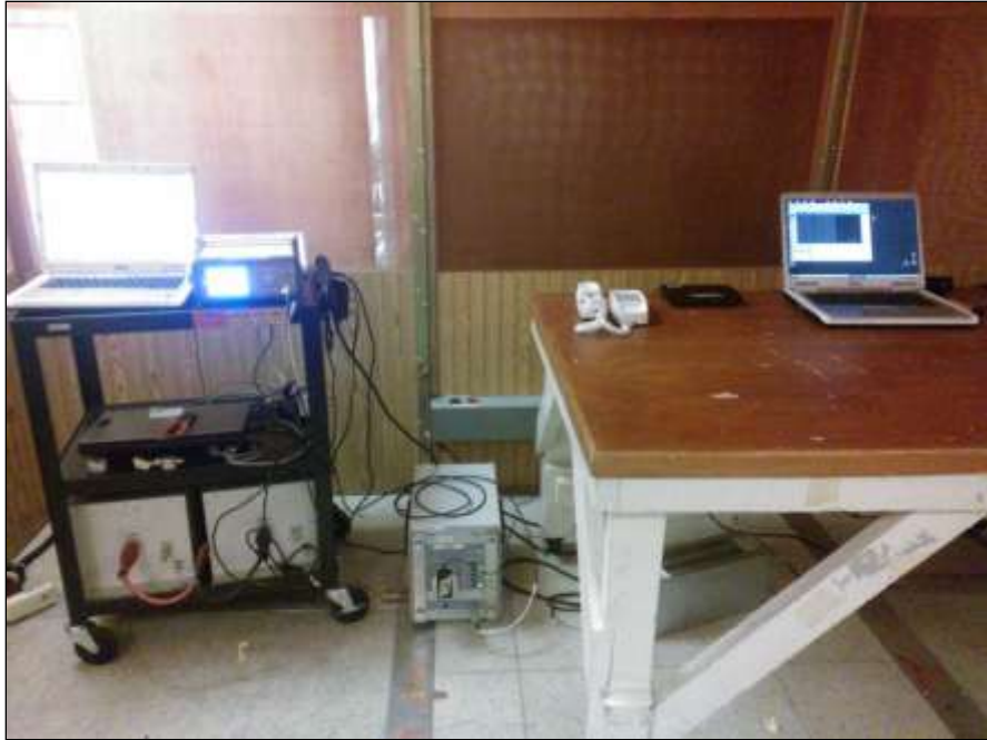
Photograph 1. Conducted Emissions, Test Setup, Schmidt
