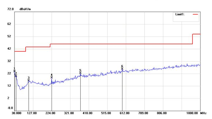
Condition: FCC Part15 RE-Class B\_30-1000MHz Polarization: Horizontal
