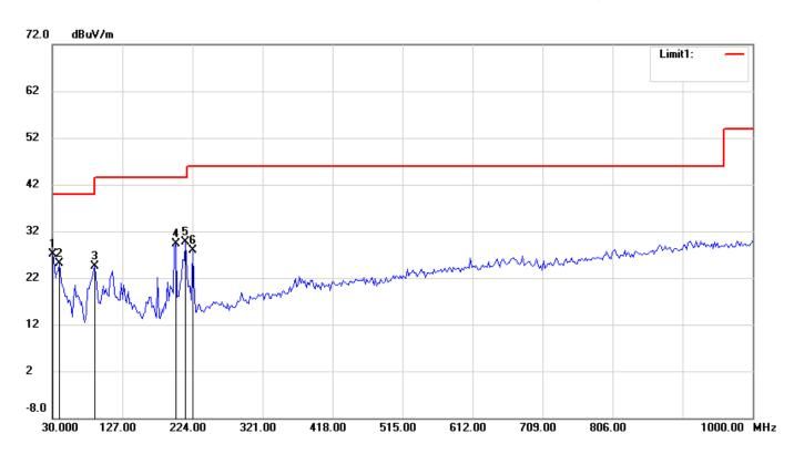
Condition: FCC Part15 RE-Class B\_30-1000MHz Polarization: Vertical
