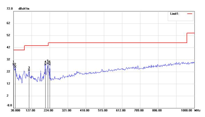
Condition: FCC Part15 RE-Class B\_30-1000MHz Polarization: Vertical
