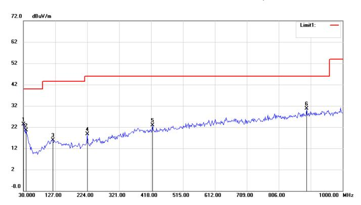
Condition: FCC Part15 RE-Class B\_30-1000MHz Polarization: Horizontal
