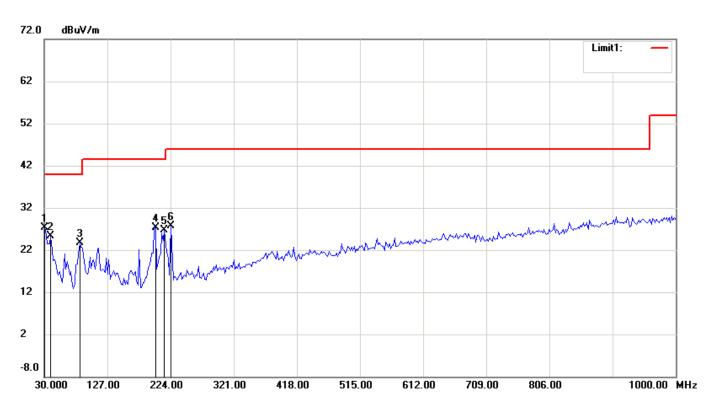
Condition: FCC Part15 RE-Class B\_30-1000MHz Polarization: Vertical
