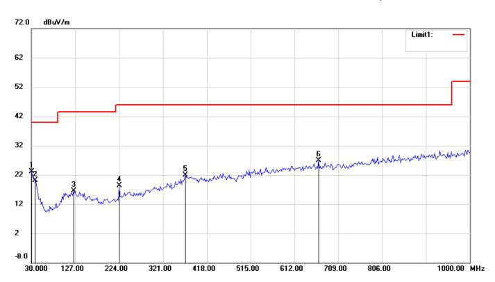
Condition: FCC Part15 RE-Class B\_30-1000MHz Polarization: Horizontal
