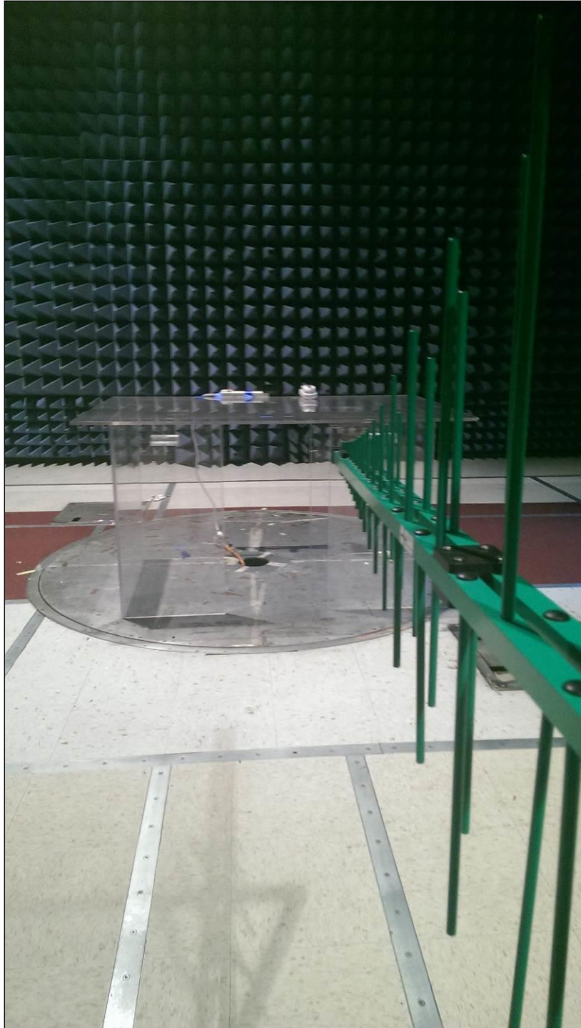
Photograph 2. Radiated Emission, Test Setup
